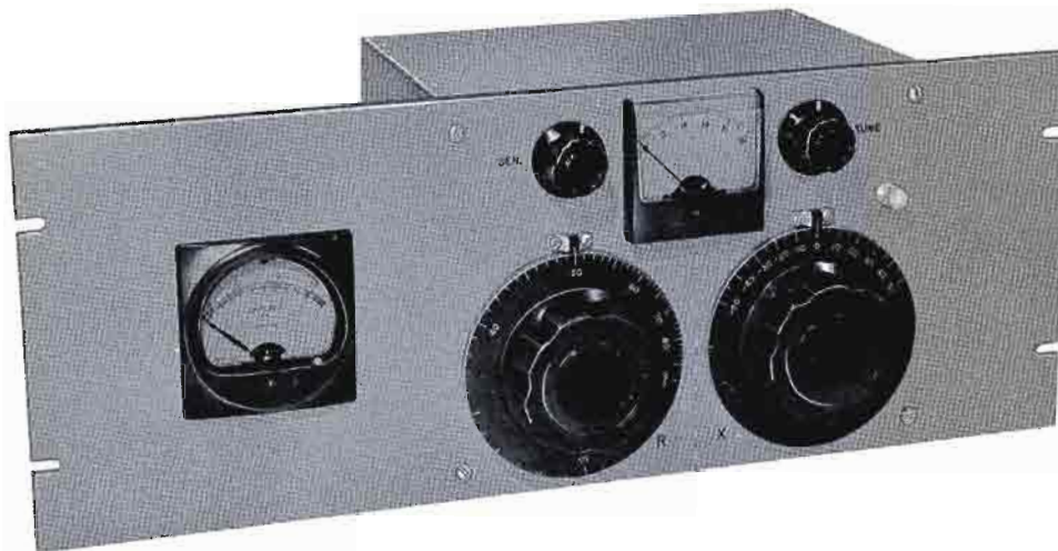
An instrument for permanent installation in the common point of a directional antenna system. Permits the common point resistance and reactance to be measured during normal operation without transmitter shutdown. Panel ammeter reads common point current so that direct antenna power can be determined.
