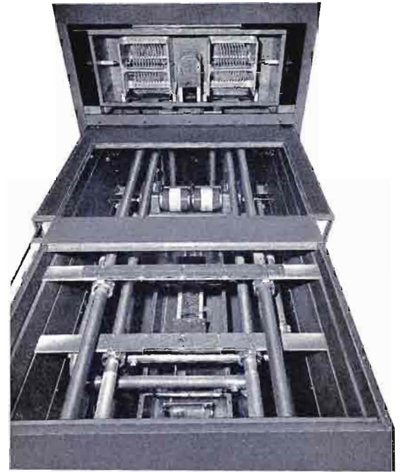
Power amplifier section with top cover removed showing the single continuously tuned line tank and separate tuned line output circuits. Note the accessibility and ease of service due to the excellent mechanical arrangement.
