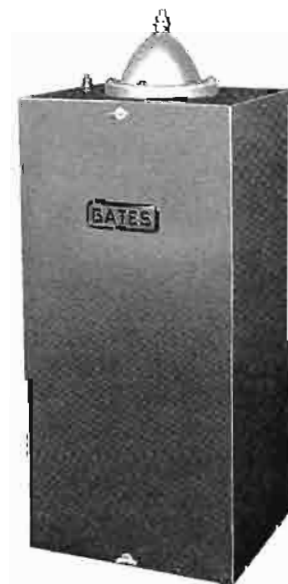
The Model M-5178 antenna coupler matches 50 ohm output of transmitter to antennas of wide variety—either vertical or long wire. It consists of edgewound coil with clips and wide range of fixed capacity in an L or TEE arrangement. The coupler may be mounted up to several hundred feet from transmitter by use of RG11U coaxial cable. Size: 21" high, 10" wide, 9" deep.
