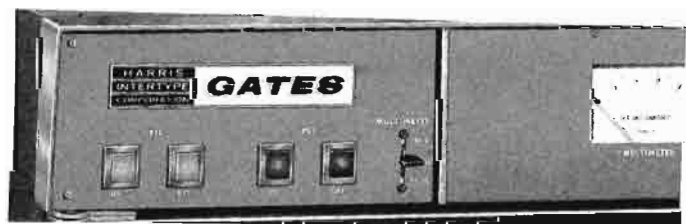
On-Off and multimeter switching functions are located on the top front panel of the FM-10G transmitter.
