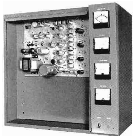
Front view (cover removed) of Model BFE-10C, ten watt FM transmitter. Models BFE-50C and BFR-50C are essentially identical in appearance.
