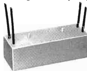
View of encapsulated amplifier. After thorough quality check, the amplifier is sealed then thoroughly tested to specifications.
