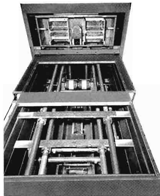
Power amplifier section with top cover removed showing the single continuously tuned line tank and separate tuned line output circuits. Note the accessibility and ease of service due to the excellent mechanical arrangement.
