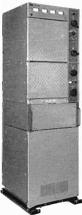
3 KW Amplifier, model HFL-3000
