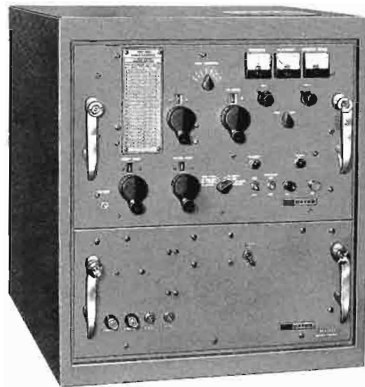
1 KW Amplifier, model HFL-1000
