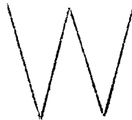
Fig. 9, Typical Waveform, Output V104 (first section)
