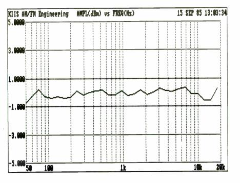
Figure 1. The record/playback frequency response of the CTR-100. The vertical axis is scaled in decibels; the horizontal axis in frequency.
