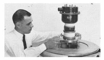
Figure 16—Adjustment of Prefocus Coil.
