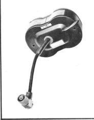
The linear tuning characteristics of this magnetron simplifies programming the frequency sweep, by eliminating the complicated compensating networks required by other voltage tunable oscillators.
