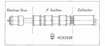
Figure 4—Typical Eimac Externally Tuned Klystron, Compared to a 250-Watt UHF Tetrode Tube.
