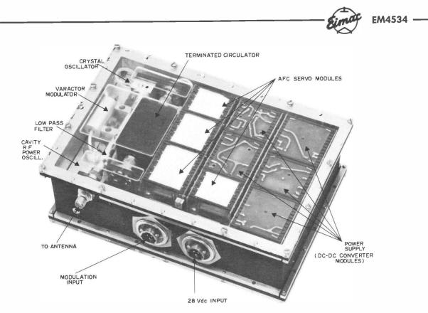
EM4534 TELEMETRY TRANSMITTER ASSEMBLY
