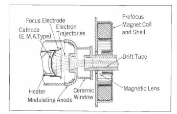
Figure 5—Simplified View of Electron Gun, Prefocus Magnet Coil and Entrance to Drift Tube.
