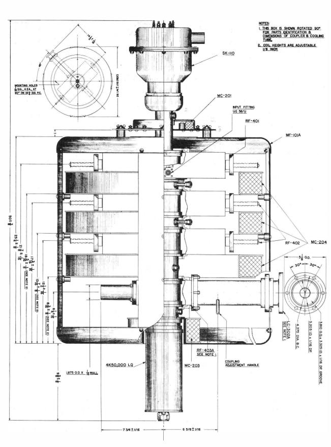
H-101A KLYSTRON AMPLIFIER CIRCUIT ASSEMBLY
