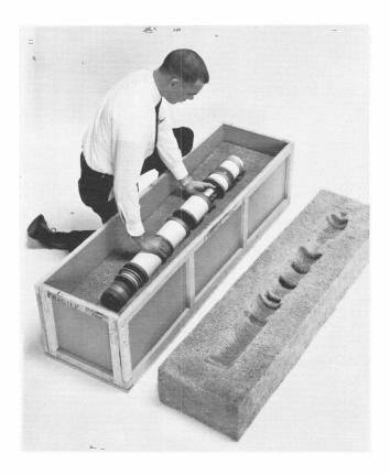
Figure 10—Storage of Klystron in Shipping Crate.
