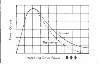
Figure 17—Overdriving a Klystron Reduces Output.
