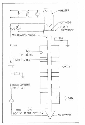
Figure 20—Klystron Power Supply Connections
