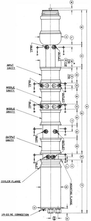
DIMENSION DATA MAX. MIN. REF NOM. 44.560 44.690 A 7.470 7.510 B 4.985 5.040 C 20.064 19.994 D .626 E 12.620 F 12.515 3.530 G 3.495 1.205 н 1.170 .255 J .230 1.100 ĸ 1.030 L .515 .645 Μ .187 N .750 Ρ .560 .650 Q 2.735 2.770 4.630 D R 4.610 D 4.510 D 4.490 D **\$** T 1.320 1.425 5.130 D U 5.115 D 4.640 D 4.610 D ٧ Х 2.120 2 140 Y .645 .705 AB 1.585 1.630 AC 60\* AD 30° AE 3.485 3.510 AF 1.875 AG 4.000 AH 2.563 AJ 4.615 4.635
