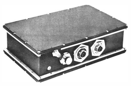
Model EM4534 is a complete transmitter, including a pre-regulated DC-DC converter. All circuits are solid state, except the rf power oscillator, which is a single stage rugged ceramic planar triode. RF is generated at the output frequency. The complete transmitter package displaces less than 50 cubic inches, and weighs 4.5 pounds. Major features of this transmitter include:
