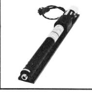
The EM-1050 features rugged ceramic and metal construction and focusing is provided by built-in periodic permanent magnets. These magnets are fully temperature compensated to allow operation from -55 to  $+85^{\circ}$ C. No additional cooling is required at these temperatures due to the integral heat sink/mounting flange supplied with the tube.
