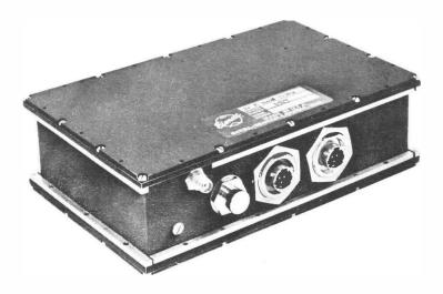
Model EM 4527 is a complete transmitter, including a pre-regulated DC-DC converter. All circuits are solid state, except the rf power oscillator, which is a single stage rugged ceramic planar triode. RF is generated at the output frequency. The complete transmitter package displaces less than 50 cubic inches, and weighs 4 pounds. Major features of this transmitter include:
