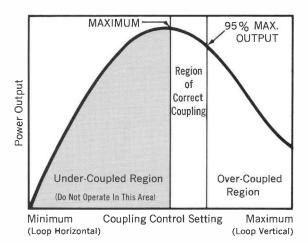
Figure 19-Adjustment of Output Coupling Control.
