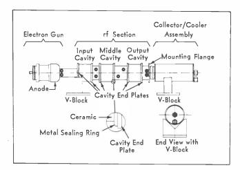
Figure 12—View of Klystron Mounted Correctly on V-Blocks.
