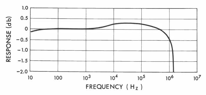
TYPICAL MODULATION FREQUENCY RESPONSE OF TRANSMITTER
