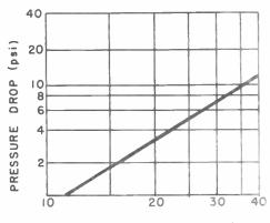
COLLECTOR WATER FLOW (gpm)
