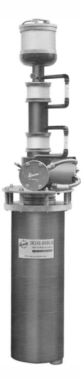
Eimac 3K210,000LQ. This 75 kW klystron is used in many tropo-scatter systems spanning distances up to 440 miles. This klystron is unique in that its input and penultimate cavities are external but its output cavity is integral.
