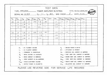
Figure 14—Test Data Card. (front)
