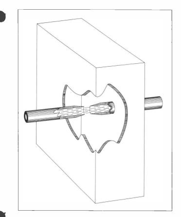
Figure 6—Simplified View of Resonant Cavity. Note Drift Tube Tips. Electron Trajectories Represented by Broken Lines.
