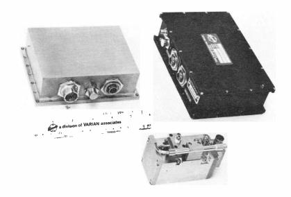
Model X4528 is a complete transmitter. It includes an exciter, a power amplifier and a preregulated dc-dc converter. All circuits are solid state, except the rf power oscillator and the power amplifier; these use rugged ceramic planar triodes. RF is generated at the output frequency, and stabilized by a crystal-referenced AFC servo circuit. Major features of this transmitter include:
