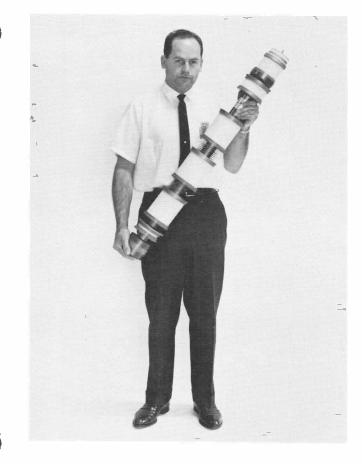
Figure 11—Recommended Method of Hand Carrying Eimac Klystrons.
