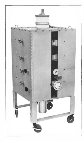
Figure 8—4KM100LA Klystron and H-163 Circuit Assembly. Designed for UHF Television, This Tube Develops 25 Kilowatts of Peak Synchronizing Power at Frequencies from 470 to 610 Megacycles.
