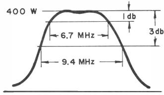
DRIVING POWER - 500 mW OUTPUT POWER - 400 W GAIN - 29 db EFFICIENCY - 35 % I db BANDWIDTH - 6.7 MHz 3 db BANDWIDTH - 9.4 MHz
