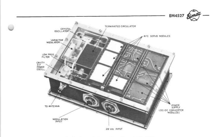
EM4527 TELEMETRY TRANSMITTER ASSEMBLY
