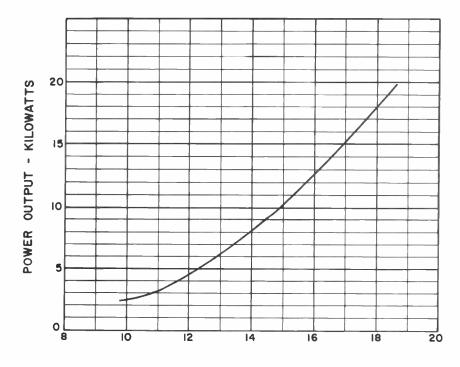
D-C BEAM VOLTAGE - KILOVOLTS
