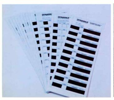
CARTSCAN labels are preprinted on adhesivebacked thin-film Mylar® An appropriate label is selected and affixed to the right edge of each cartridge prior to recording. Optically coded reflective areas of the label are read by infrared sensors in the DYNAMAX CTR100 Record and Playback machines. CARTSCAN labels automatically switch the CTR100 to the preselected format. Unlabeled cartridges are recorded and played normally.
