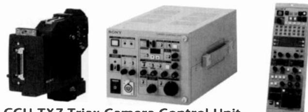
**CCU-TX7 Triax Camera Control Unit**
