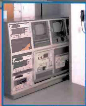
**A Four Bay Corner Console.** 14" Slope racks for decks and edit control equipment. Three upper 10-1/2" monitor racks tilted forward for effortless viewing. One upper vertical rack for a VTR. 18"D Dove Grey work surface with accent contour trim. Pearl Grey and Dove Grey enamel finish.
