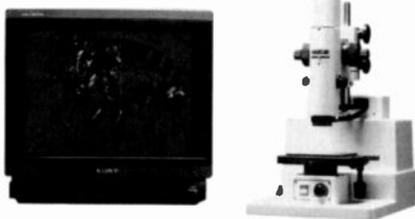
objects from 23mm down to 70 microns ■ Built-in high resolution color CCD camera, fiber optic illumination system, stand, stage and precision optics ■ Magnification range is 14X-371X in macro mode or 70X-4377X in micro mode using a 13" monitor ■ Continuous zoom lens
