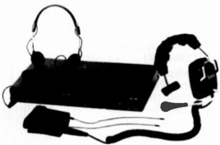
The lightweight (13 oz.) belt-pack transceiver was designed to be water-resistant and withstand abusive industrial applications. It features simple push-to-talk operation with handy low battery and overmodulation indicators. It has an impressive 24-hour battery life using 6 alkaline "AA" batteries. By using "AA" rechargeable NiCad batteries, 8 hours of use can be expected.
