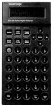
**Data Format Analysis** Reports data errors, including line/field length, illegal vertical interval switch, EAV/SAV format, illegal data values, ANC packet format and missing data bits.
