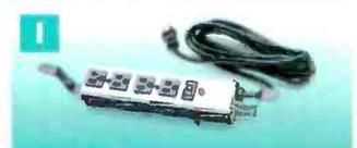
**I Electrical Assembly.** Bolts to the side of the leg on the console frames. Four outlets with circuit breaker, master switch, pilot light, 15' 3-wire cord and mounting bracket.
