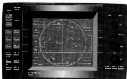
**TVM-621 Combination Waveform Monitor/Vectoroscope**
