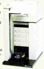
troller; every aspect of operation is software controllable. Front panel controls allow manual operation of the Reject drawer, the Input/Output drawer, and the robotic'picker." Sensors verify disc position to insure smooth operation and gentle disc handling.
