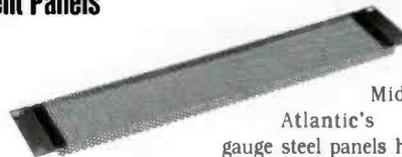
Middle Atlantic's 16 gauge steel panels have one piece construction and are perforated with 5/32" diameter holes yielding 68% open area.
