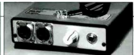
For a self contained headphone amp, we offer the IFA-7. Separate left and right XLR inputs ease installation. Requires PS-1 power supply.
