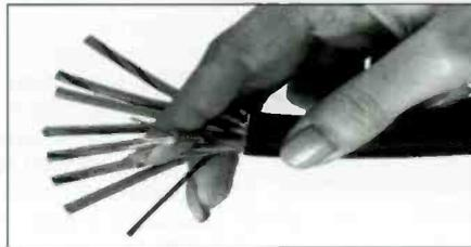
Star Quad gets its name from the four-conductor style construction that minimizes the "loop area" between twists of the conductors, reducing susceptibility to noise. It's designed for use with mics but is also excellent for all line-level signals. Buy it by the foot or in two reel sizes.
