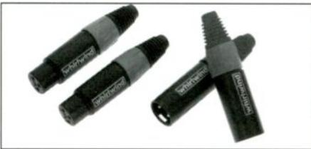
Beautiful XLR's for inline applications. Whirlwind's WI series features one piece, die cast housings, and 100% cable strain relief. Use with cable diameters from 0.11" to 0.31". Strain relief boots are black, with red, blue, and white available by special order.
