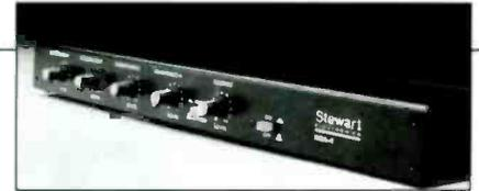
It'll feed headphones of 8 ohms to 2,000 ohms. Response is 20Hz to 20kHz, ±0.5dB. Connectors are 1/4" TRS.
