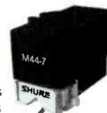
The popular M44 Series models feature a spherical diamond stylus (0.7 mil) with a large-diameter stylus assembly. Tracking force specs are as follows: M44G .75 to 1.5 grams; M447 1.5 to 3 grams. The SC35C features a spherical diamond stylus (0.7 mil) with a large-diameter stylus assembly. Tracking force is 4 to 5 grams.
