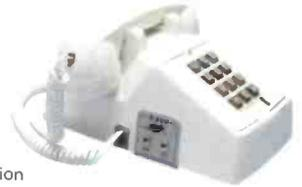
TAC and TAC+ are inserted between the handset and handset jack on the telephone. TAC provides a switch to match input levels and also a mute switch for the handset mic. TAC+ adds a momentary mic mute (cough) and selector switches for different input attenuation and impedance ranges.
