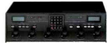
MAX-Z is a remote broadcast console providing flexibility and excellent audio quality. Features: 4 XLR mic/line inputs; front panel level and rear panel gain controls; cue buttons on channels 1 and 4; monitor input (mini jack) feeds into the cue channel; phone line out; direct audio out; 4 headphone jacks; built-in rechargeable batteries or AC power; VU meter; telephone keypad; carrying case.
