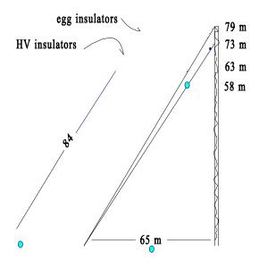
when you do this). When the self resistance no longer drops significantly with increasing radials, you have a good compromise. Keep in mind that the existing radials from the tower can assist, and may be brazed to the new radials where they intersect.
