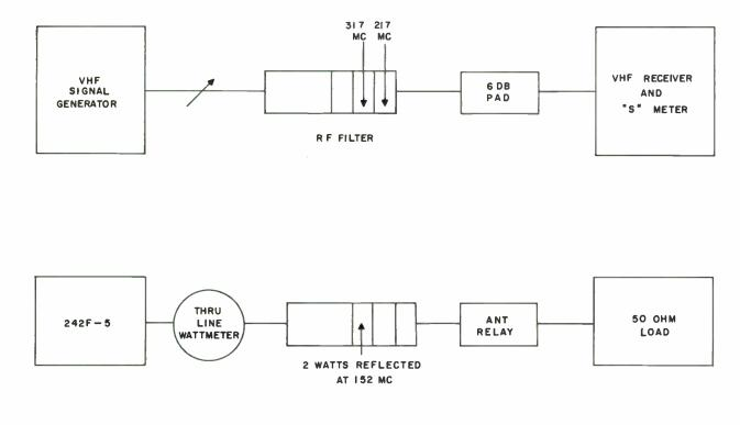
Figure 6-9. R-F Low-Pass Filter Adjustment and Tuning Test Setup
