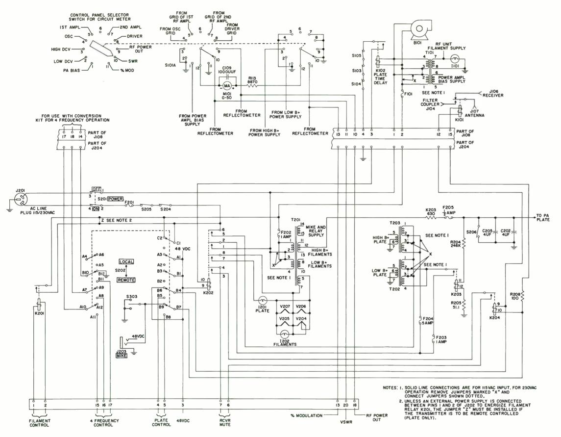
Figure 4-10. Control Circuits
