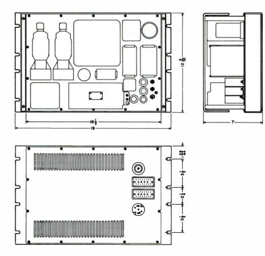
Figure 2-3. Modulator-Power Supply, Midrail Installation Diagram
