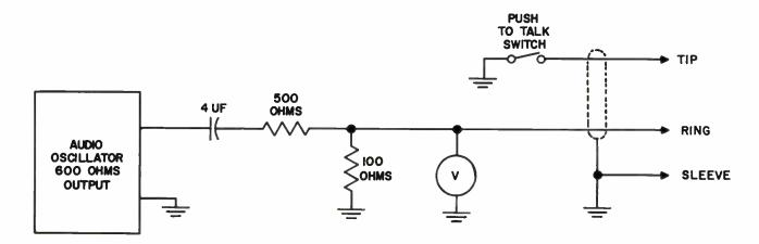
Figure 6-8. 82-Ohm Dummy Carbon Mike for Percent Modulation Meter Calibration, Test Setup
