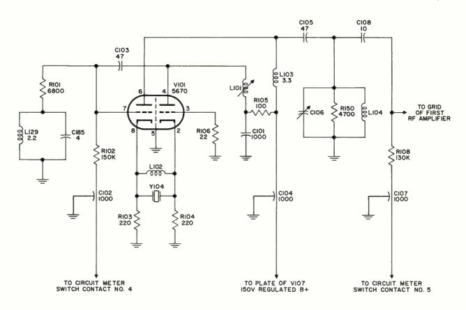
Figure 4-2. Oscillator-Frequency Doubler
