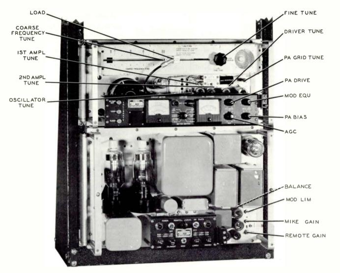
Figure 2-8. Tuning and Adjustment Controls
