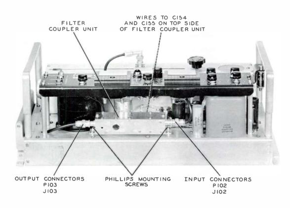
Figure 6-5. R-F Unit, Bottom View Showing Filter Coupler Unit
