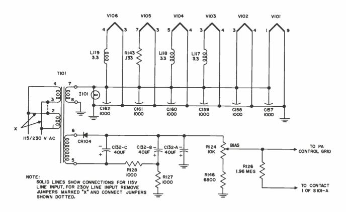
Figure 4-7. R-F Filament and Power Amplifier Bias Power Supplies
