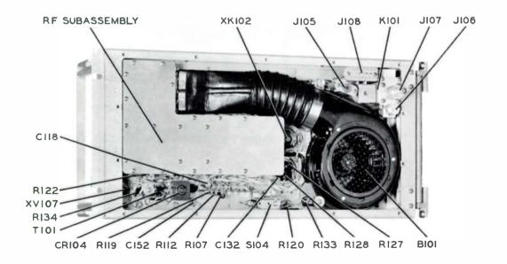
Figure 7-3. R-F Unit, Rear View, Dust Cover Removed
