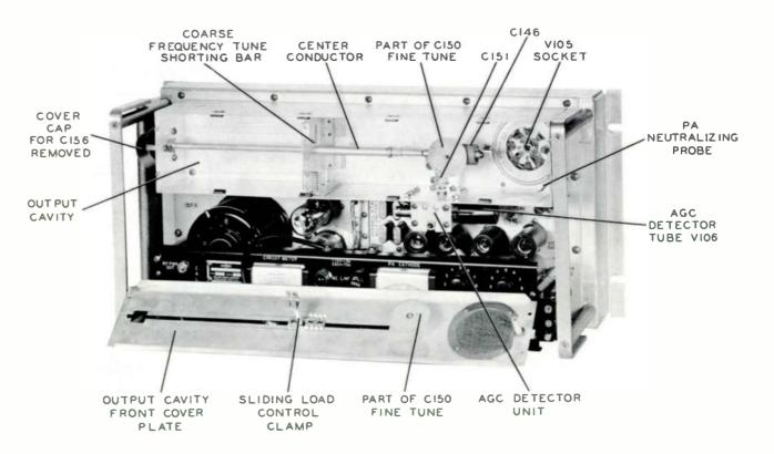
Figure 6-3. R-F Output Cavity Disassembled
