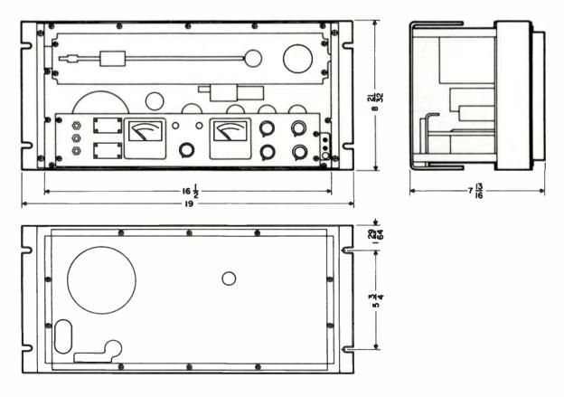
Figure 2-2. R-F Unit, Midrail Installation Diagram
