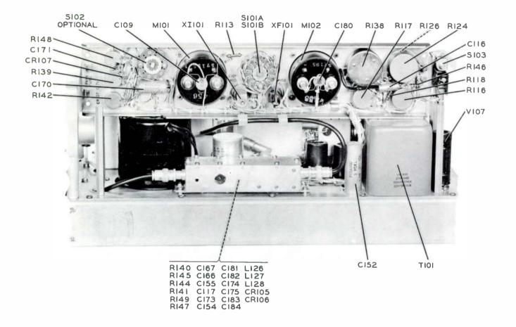
Figure 7-2. R-F Unit, Bottom View, Dust Cover Removed, Back View of Control Panel
