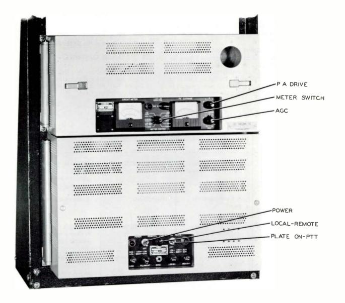
Figure 3-1. VHF Transmitter 242F-5CL, Operating Controls
