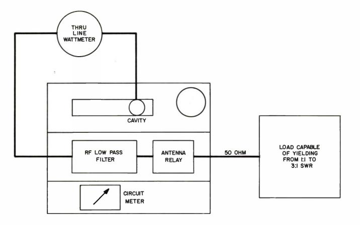
Figure 6-6. R-F Power Out and VSWR Indicators, Calibration Test Setup
