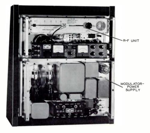
Figure 2-1. VHF Transmitter 242F-5CL, Hinge Mounted
