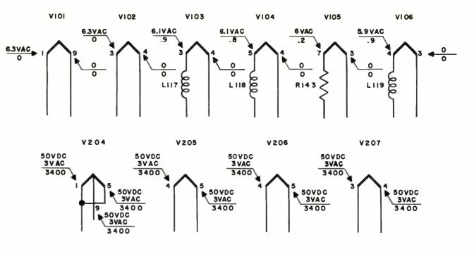
Figure 6-2. Filament Voltage and Resistance Measurements
