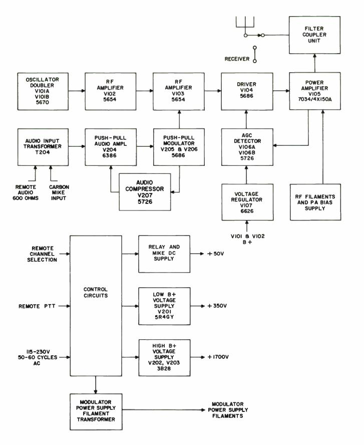
Figure 4-1. VHF Transmitter 242F-5CL, Block Diagram
