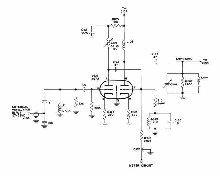
Figure 4-12. External Oscillator Modification
