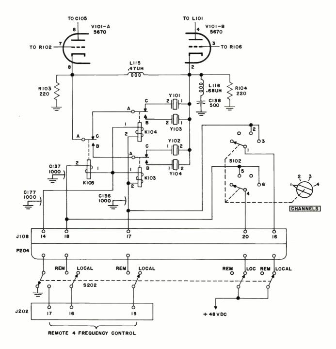
Figure 4-11. Four-Frequency Modification
