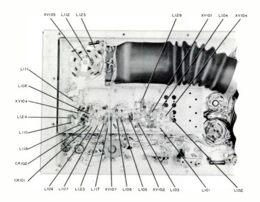
Figure 7-5. R-F Unit Subassembly, Cover Plate Removed
