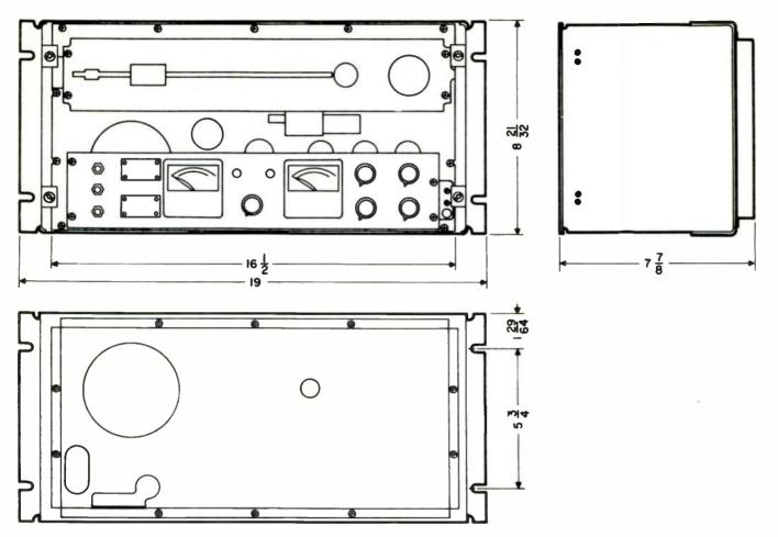
Figure 2-4. R-F Unit, Flush Mounting Installation Diagram
