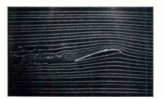
Symmetrical section with angle of attack. Controls allow demonstration of attack angle transition from zero angle to vertical.
