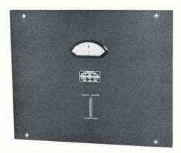
1181-B FREQUENCY DEVIATION MONITOR — Gives direct indications of magnitude and direction of frequency deviation of AM transmitter. Positive indication is provided for failure of either transmitter carrier or monitor crystal oscillator. Frequency Range: 0.5-2 mc (specify crystal frequency). Deviation Range: ± 30 cps. Primary Power: 105-125 or 210-250 v, 50/60 cps, 125 watts. Size: 19" W, 13" D, 15¾" H. Weight: 51 lbs.
