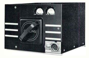
180M-1 ANTENNA TUNING UNIT TEST SET — A manually adjustable network used to minimize the time required to determine the circuit elements which must be wired into the 180K-3. Circuits and values of capacitance and inductance selected by front panel controls. Size: 73/4" H, 101/4" W, 97/8" L.
