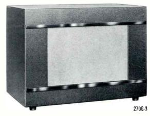
**270G-3 CABINET-SPEAKER** — This unit consists of cabinet and 10" PM speaker, 6-8 ohm impedance voice coil, 8 watts. It is attractively finished to match 51J-4 and 75A-4 Receivers. Size: 15" W,  $9\frac{1}{8}$ " D and  $10\frac{5}{8}$ " H. Weight:  $12\frac{1}{2}$  lbs.
