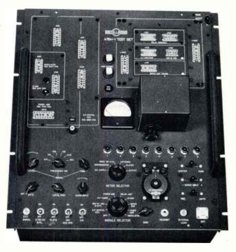
478H-1 618S TEST SET — The 478H-1 and associated 413F-1 Power Supply provide complete self-contained facilities for testing modular subassemblies of the 618S. Also provides a convenient test station for detailed circuit checks. The lower portion of the test set panel carries all operating controls required to simulate functions of the complete 618S Transceiver. *Weight:* 35 lbs. *Size:*  $19\frac{1}{52}$ " H,  $17\frac{1}{2}$ " W, 8" D.
