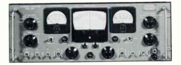
477N-1 STEERING COMPUTER TEST SET — Simulates selected heading, bank and course datum signals normally supplied to the 562A-5 Steering Computer. All important circuit functions may be tested and adjustments implemented. Complete test takes 15 min. Rack mounting.
