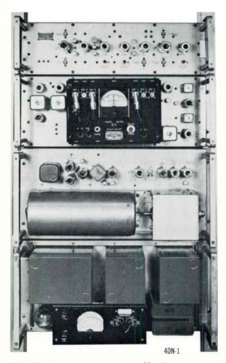
40N-1 FREQUENCY STANDARD — May be used in applications requiring extreme stability of mixing injection frequencies in both transmitting and receiving equipment. It consists of the 40K-1 High Stability Oscillator and associated 426A-1 Power Supply, 8U-1 Frequency Divider and 54M-1 Frequency Comparator. The 40N-1 may also be utilized as a secondary frequency standard.
