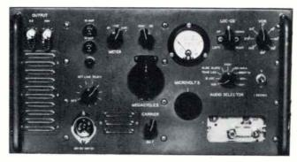
479T-2 ALL CHANNEL VOR-ILS SIGNAL GENERATOR — A portable test set for ramp testing of navigation and ILS receivers. May be used inside or outside the plane for an over-all check on the installation from receiving antenna to indicating instruments. Complete coverage of all channels from 108.0 through 135.9 and 329.3 through 335.0 mc. RF level can be varied from 4 to 200,000 microvolts. Signals include: VOR, LOC, glideslope, 1000 cps audio tone. Size: 19" W, 18" H,  $10\frac{1}{2}$ " D.
