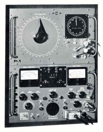
477U-1, 477V-1 ADF TEST SET — Provides complete test and simulator signals for the DF-201 ADF. The 477U-1 ADF Loop Simulator generates a calibrated RF field and excites a contained loop antenna. Receiver bearing indications are displayed on the front panel. The 477V-1 tests antenna, loop, ADF aural and ADF bearing sensitivity, dial calibration, hearing speed, AVC and gain control characteristics, and makes test point measurements on individual modules. *Mounting:* Rack or carrying case.
