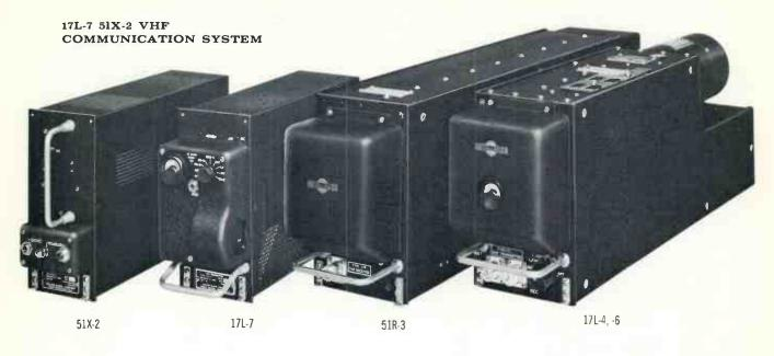
**51R-3 VHF COMMUNICATION/NAVIGATION RECEIVER** — A 280 channel crystal-controlled receiver with 100 kc spacing between 108.0 and 135.9 mc. Receives all VOR/LOC and communication frequencies and with the accessory frame and accessories provides full instrumentation facilities. *Shockmount:* 350E-3A. External power supply required.
