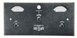
1931-B AM MODULATION MONITOR — Measures percentage modulation on positive or negative peaks, indicates overmodulation, monitors program level and measures transmitter audio frequency response and carrier shift when modulation is applied. Operates in 0.5 to 8 mc range. *Primary Power:* 105-125 v, 50/60 cps, 50 watts. *Size:* 19" W, 10" D, 8¾" H. *Weight:* 32 lbs.
