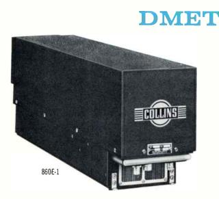
Collins 860E-1 Distance Measuring Equipment, TACAN, provides precise distance information for aircraft up to 200 nautical miles from an associated ground beacon. The power amplifier provides 1 kw minimum peak pulse power.
