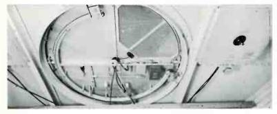
Above. Convenient access to antenna interior is through screened hatch. The eight point bearing check may be made without leaving the house by turning the outer shell with crank supplied.
