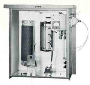
42E-7, -8 ANTENNA COUPLING UNITS — Use a low pass T network to match a series fed vertical radiator to an unbalanced transmission line. The 42E-7 (pictured) is used up to 1 kw; the 42E-8, 5 or 10 kw. Includes antenna current meter and line current meter jack and will house tower lighting filter choke and antenna current transformer. Size: 42E-7 29" W, 18" D, 28" H. 42E-8 — 36" W, 22" D, 28" H. Weight: 42E-7 — 64 lbs. 42E-8 — 124 lbs.
