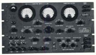
478C-2 FD-104 IFS TEST SET — Provides accurate simulated aircraft heading signals, lateral and vertical displacement signals, attitude signals, and rate of change of these signals as necessary for bench testing and calibrating the Collins 562A Steering Computers and components of the FD-104 IFS. Provides .001 to 10 cps signals for testing meter responses and servo mechanisms. No vacuum tubes are used. *Power Requirements:* 230 watts max. *Size:* 10<sup>1</sup>/<sub>2</sub>" H, 19" W, 12" D.
