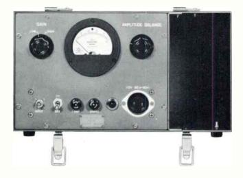
478A-1 ZIFOR (Zero Indicator for Omni-range) — Used for precisely ascertaining the proper zero, or North, setting on audio signal generators used in VOR testing and to set the zero on the Collins 479S series of test equipment or their equivalents. May also be used to check for phase shift through the RF signal generator. Used with the 479S-3. Size:  $13\frac{1}{2}$ " H,  $13\frac{1}{2}$ " W,  $7\frac{1}{2}$ " D.
