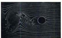
Airflow around a cylinder with KARMAN street vortices in the wake. High speed lighting is necessary for stop motion photography.
