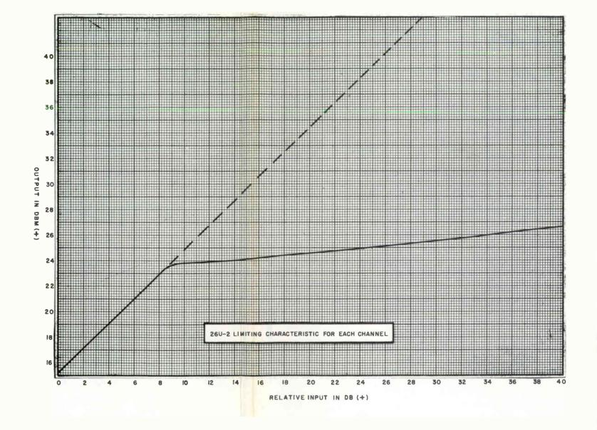
Figure 1-3. 26U-2 Stereo Peak Limiter, Limiting Characteristic Curve
