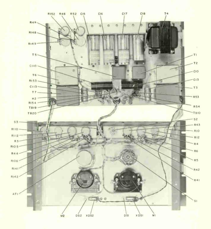
Figure 6-6. 26U-2 Stereo Peak Limiter, Module Separated at Center
