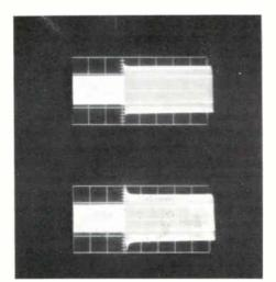
Figure 5-2. 26U-2 Stereo Peak Limiter, Attack Time
