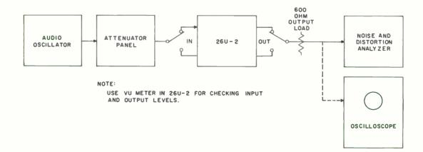
Figure 5-1. Test Setup, Block Diagram
