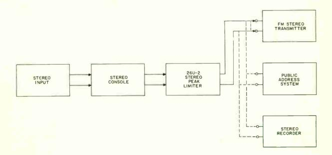
Figure 1-2. 26U-2 Stereo Peak Limiter, Application Block Diagram
