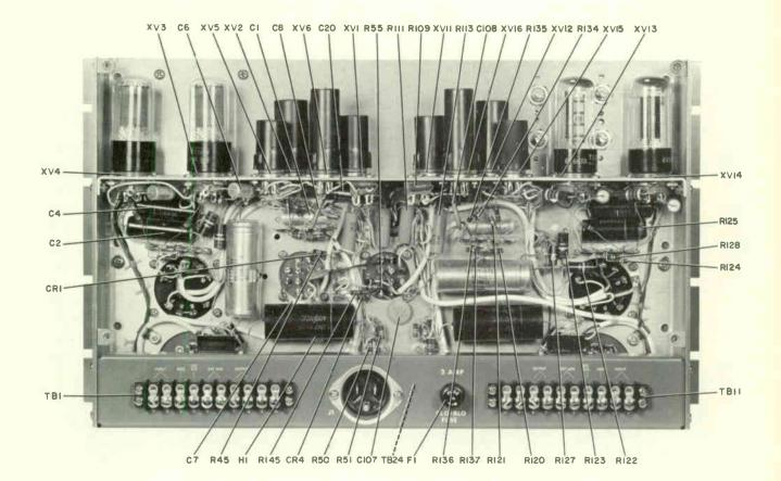
Figure 6-2. 26U-2 Stereo Peak Limiter, Inside Back View
