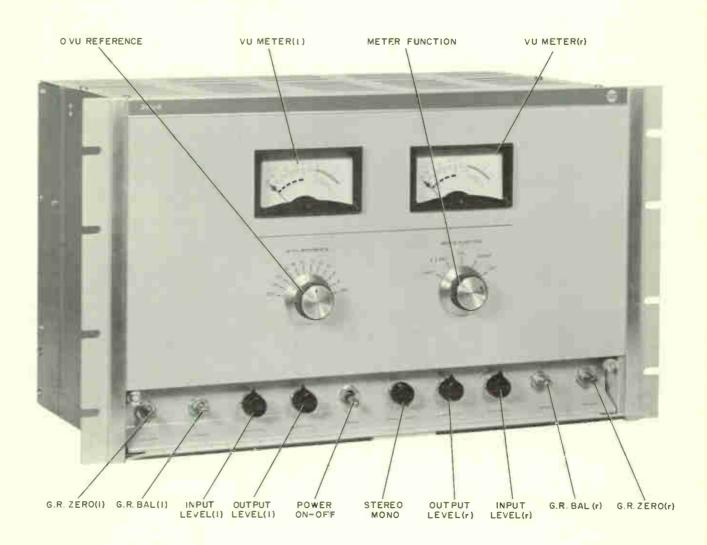
Figure 3-1. 26U-2 Stereo Peak Limiter Operation Controls, Front View
