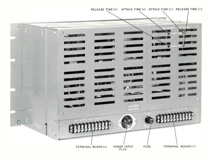
Figure 3-2. Operational Controls, Rear View
