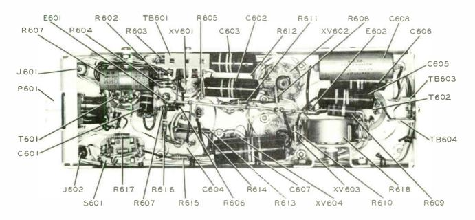
Figure 10. Limiter Amplifier, 356E-1 Bottom View
