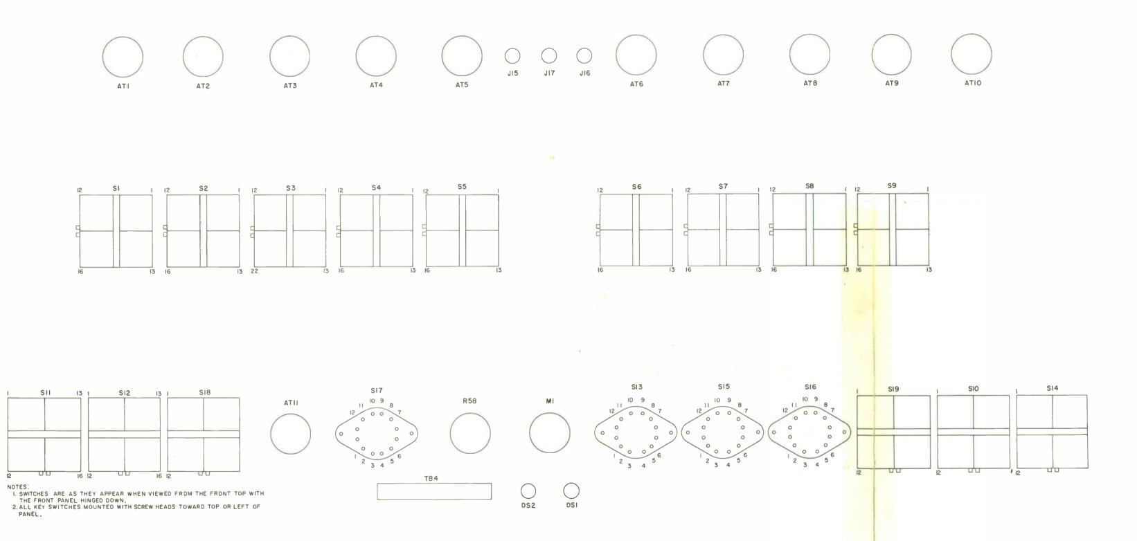
Figure 7-2. Broadcast Console 212G-1 Switch Pin Orientation
