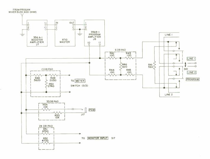
Figure 4-3. Program Circuits, Simplified Schematic Diagram
