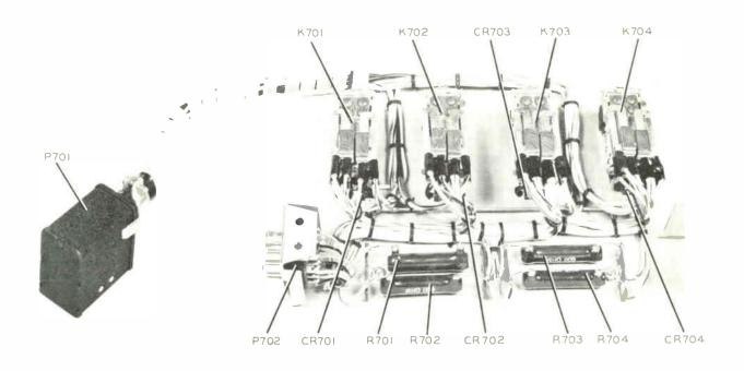
Figure 2. Relay Unit 274K-2, Cover Removed
