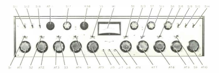
Figure 3-1. Broadcast Console 212G-1, Control Locations
