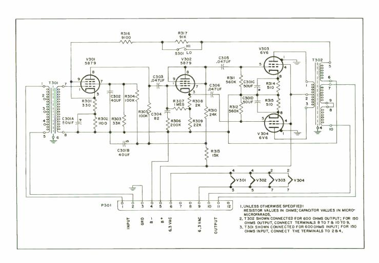
Figure 4. Program/Monitor Amplifier, 356B-1, Schematic Diagram
