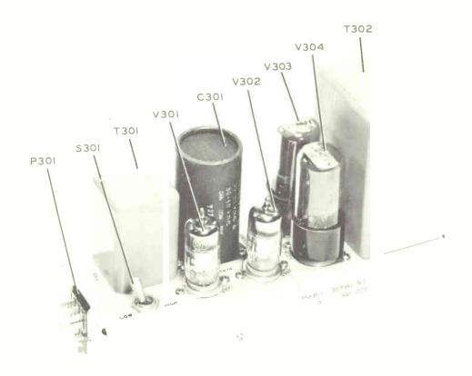
Figure 2. Program/Monitor, Amplifier, 356B-1, Top View
