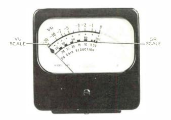
Figure 7. Vu Meter With GR Scale Decal Applied
