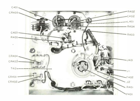
Figure 2. Power Supply 409X-2, Bottom View
