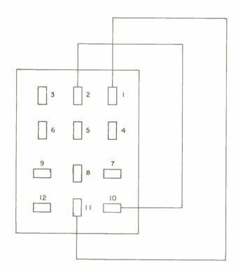
Figure 2-3. Jumper Plug Wiring Schematic Diagram
