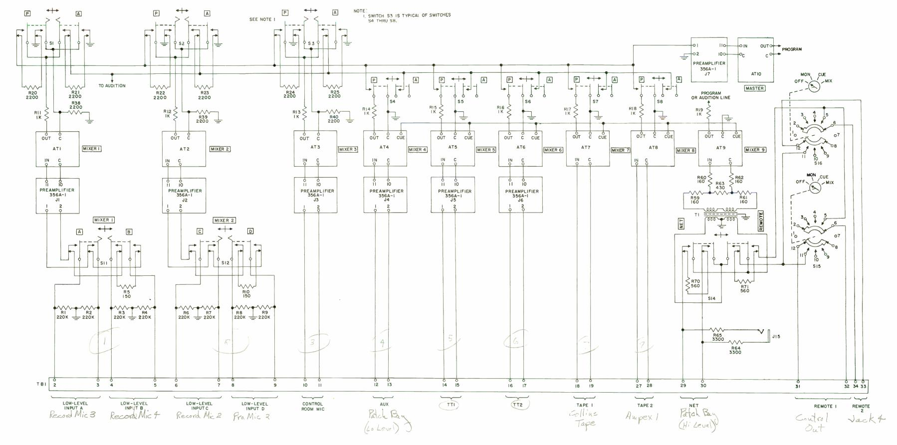
Figure 4-2. Mixer Circuits, Simplified Schematic Diagram
