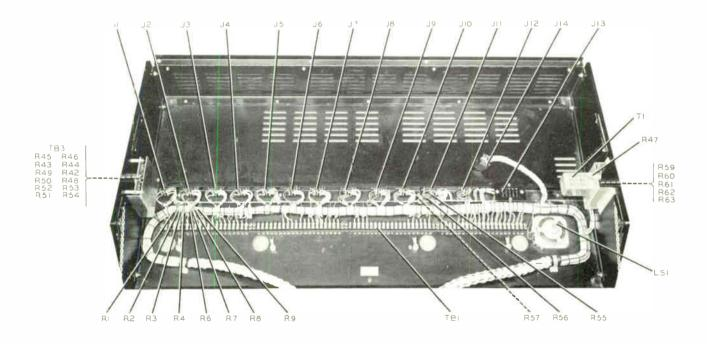
Figure 6-2. Broadcast Console 212G-1, Inside View
