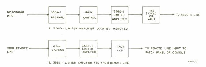
Figure 3. Collins Type 356E-1 Limiter Amplifier as Automatic Level Control, Suggested Arrangement
