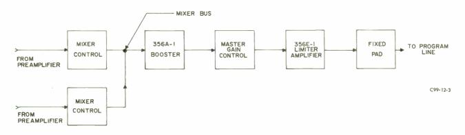
Figure 4. Collins Type 356E-1 Limiter Amplifier as Automatic Mixer,
