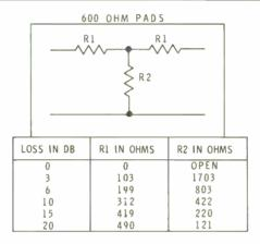
Figure 2-4. Resistor Values for Fixed Pads
