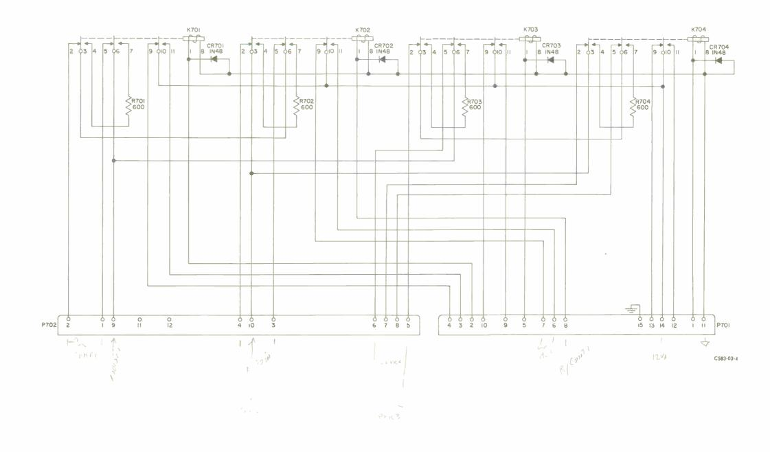
Figure 3. Relay Unit 274K-2, Schematic Diagram
