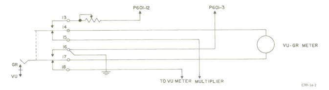
Figure 8. Vu Meter and GR Switch Connections, Schematic Diagram
