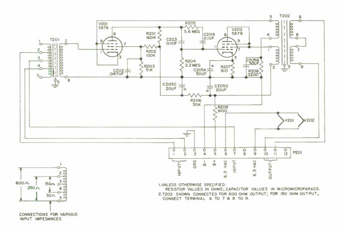
Figure 4. Preamplifier 356A-1, Schematic Diagram
