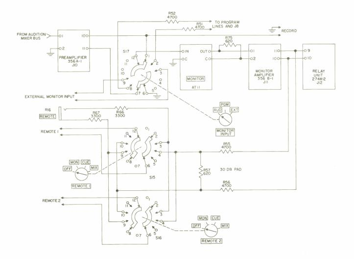
Figure 4-4. Monitor Circuits, Simplified Schematic Diagram
