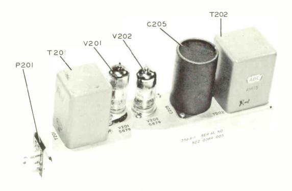
Figure 2. Preamplifier, 356A-1 Top View
