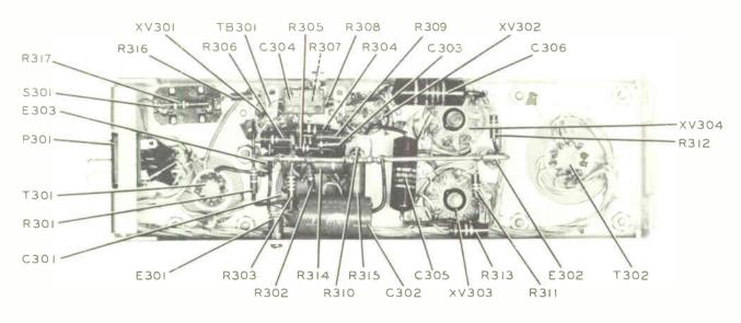
Figure 3. Program/Monitor Amplifier, 356B-1, Bottom View
