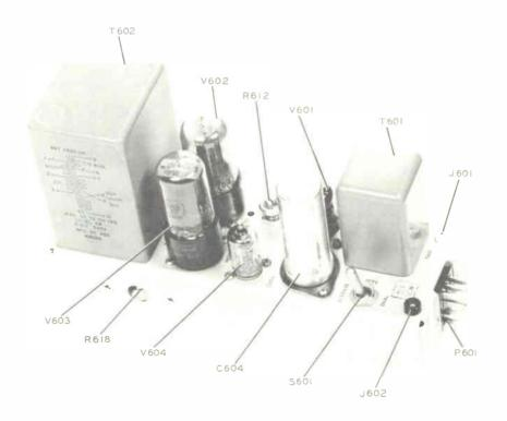
Figure 9. Limiter Amplifier, 356E-1 Top View
