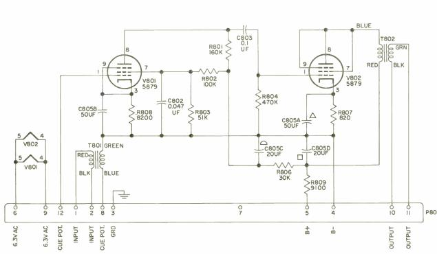
Figure 3. Cue Amplifier 356Q-1, Schematic Diagram
