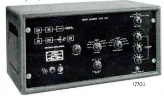
477C-1 NOISE LOADING TEST SET — The 477C-1 provides full test facilities for the determination of system intermodulation distortion of frequency division, single sideband carrier equipment. It generates a Gaussian noise test signal and measures the intermodulation noise appearing in one or more of six 12 kc notches, or stop bands, in the test signal spectrum.
