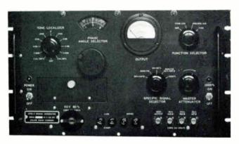
479S-3 VOR AUDIO SIGNAL GENERATOR — Used for precision testing and calibration of VOR receivers. It provides all output signals required for VOR, tone localizer and
