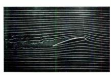
Symmetrical section with angle of attack. Controls allow demonstration of attack angle transition from zero angle to vertical.
