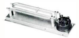
ANTENNA CURRENT TRANSFORMER—Used with remote thermocouple and meter for remote monitoring of antenna current. For currents up to 25 amps.
