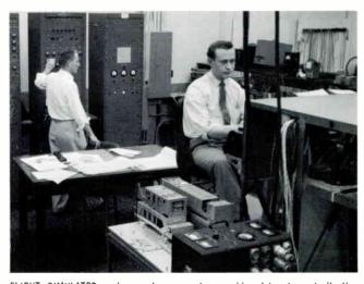
FLIGHT SIMULATOR, using analog computer, enables laboratory duplication of aeronautical conditions for analysis of airborne electronic systems.
