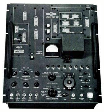
478H-1 618S TEST SET — The 478H-1 and associated 413F-1 Power Supply provide complete self-contained facilities for testing modular subassemblies of the 618S. Also provides a convenient test station for detailed circuit checks. The lower portion of the test set panel carries all operating controls required to simulate functions of the complete 618S Transceiver. Weight: 35 lbs. Size: 19 \( \frac{1}{2} \) \
