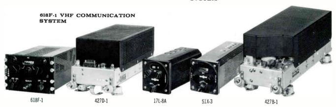
618F-1 VHF COMMUNICATION SYSTEM — The 618F-1 is a panel mounted, crystal-controlled transceiver providing 360 channel communication service with 50 kc spacing between channels in the 118.0-135.95 mc frequency range. It provides for single-channel-simplex (SCS) and double-channel-simplex (DCS) with direct frequency presentation. Only  $9\frac{\pi}{2}$  is required behind the panel, including space for rear connectors. Minimum transmitter output is six watts.
