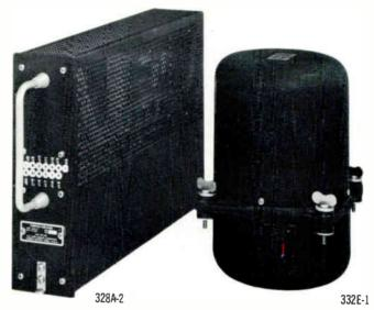
The MC-102 is a lightweight, gyro-stabilized airborne magnetic compass. The system provides  $\pm 1.0^{\circ}$  of accuracy. Initial automatic slaving at 360° per minute rapidly synchronizes the DG with the earth's magnetic field. After synchronization, the system changes to normal slaving speed of 2 to 3 degrees per minute. Power Requirements: 115 v, 400 cps, start — 88 va, run — 65 va; 27.5 v dc, start — 24 watts, run — 5 watts.
