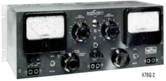
478G-2 TEST PANEL — Facilities for setting line levels of Collins carrier equipment. Includes a signal source, meters and attenuators. Test Signaling: 1000 cps, variable +10 to -28 dbm, 600 ohms. Meter Ranges: -20 to +12 dbm, 600 ohm impedance, bridging or balanced. Meter Response: Essentially flat to 2 mc for signal levels up to 3 v ac. Power Requirements: 130 v dc, 10 ma; 6.3 v, .35 amps, or 24 v. Size: 19" W, 7" H. Weight: 12 lbs.
