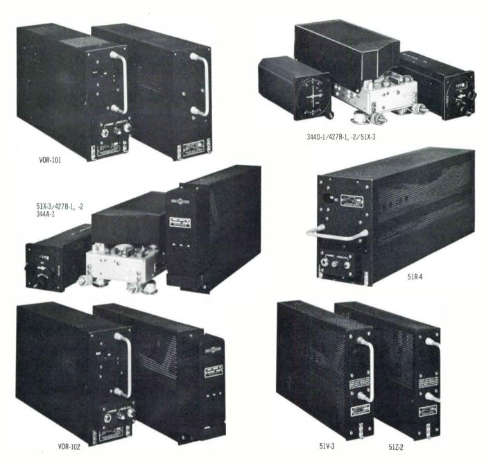
Collins Navigation Systems provide optional variation in case size, weight and degree of instrumentation. Reliability, accuracy, ease of maintenance and modular construction characterize these five system combinations designed to fit any VHF navigation need from airliner down through single engine aircraft. Units record azimuth runout error of less than  $\pm 0.5$  when tested with a precision track selector.
