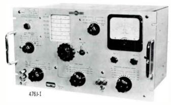
476J-1 WIDEBAND AND SELECTIVE VOLTMETER — Used to measure harmonic distortion, intermodulation products, cross-talk, attenuation and interfering frequencies of telephone carrier equipment. Wideband Voltmeter—Frequency Range: .2 to 750 kc. Voltage Range: 10 to 100 my, 1 to 10 v. Accuracy: ±5%. Selective Voltmeter—Frequency Range: 4
