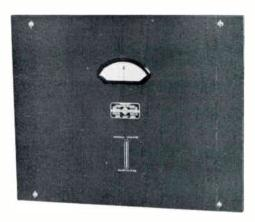
1181-B FREQUENCY DEVIATION MONITOR — Gives direct indications of magnitude and direction of frequency deviation of AM transmitter. Positive indication is provided for failure of either transmitter carrier or monitor crystal oscillator. Frequency Range: 0.5-1.6 mc (specify crystal frequency). Deviation Range: ±30 cps. Primary Power: 105-125 or 210-250 v, 50/60 cps, 125 watts. Size: 19" W, 13" D, 15¾" H. Weight: 51 lbs.
