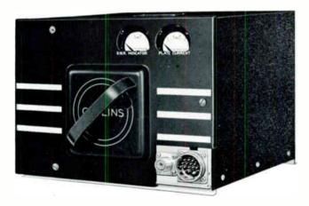
180M-1 ANTENNA TUNING UNIT TEST SET — A manually adjustable network used to minimize the time required to determine the circuit elements which must be wired into the 180K-3. Circuits and values of capacitance and inductance selected by front panel controls. Size: 73/4" H, 101/4" W, 97/8" L.
