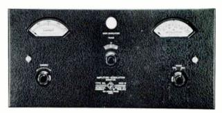
1931-B AM MODULATION MONITOR — Measures percentage modulation on positive or negative peaks, indicates overmodulation, monitors program level and measures transmitter audio frequency response and carrier shift when modulation is applied. Operates in either 0.5 to 8 mc range or 3 to 60 mc range, depending on input coil used. *Primary Power:* 105-125 v, 50/60 cps, 50 watts. *Size:* 19" W, 10" D, 8¾" H. *Weight:* 32 lbs.
