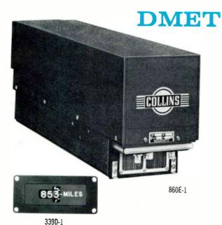
Collins 860E-1 Distance Measuring Equipment, TACAN, provides precise distance information for aircraft up to 200 nautical miles from an associated ground beacon. The power amplifier provides 1 kw minimum peak pulse power.
