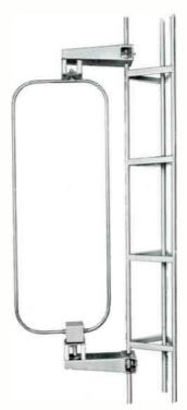
564A-1 PHASE SAMPLING LOOP — For accurate sampling of currents in directional arrays. Two loops of wire, connected in series or parallel, inside a copper tubing shield which eliminates electrostatic coupling. Connects with air or solid dielectric line. Size: Approx. 30" W, 7'6" H. Weight: 50 lbs.
