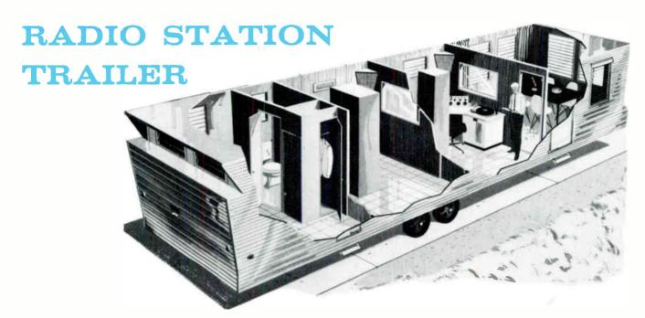
Designed as a complete radio station or mobile studio, the Collins Radio Station Trailer provides all the facilities of a permanent-type studio. All broadcast and office functions may be carried on in the four large rooms of the trailer. Large observation windows connect the studio, control room and transmitter room. Adjoining the large office is an enclosed closet and the rest room, heating and air conditioning facil-
