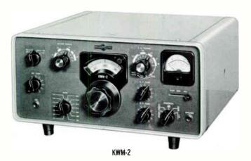
The KWM-2 Transceiver is easily moved between mobile and fixed station installations. For mobile use the transceiver slides into the mount, and the power, antenna, antenna selector and car radio speaker plugs connect automatically. These same four connectors are used in a fixed station installation.
