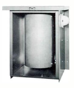
144A-1 ISOLATION COIL — Coil provides isolation for the sampling line in directional arrays, presenting a high impedance for the line across the base insulator. Unit consists of a phenolic coil form which will accommodate 37 turns of RG8/U or similar solid dielectric sampling line. May be mounted on wall of tuning shack or in 49U-1 Housing (pictured). Inductance: Approx. 180 microhenrys. Size: 10" dia., 18" L. Weight: 6 lbs.
