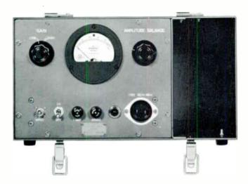
478A-1 ZIFOR (Zero Indicator for Omni-range) — Used for precisely ascertaining the proper zero, or North, setting on audio signal generators used in VOR testing and to set the zero on the Collins 479S series of test equipment or their equivalents. May also be used to check for phase shift through the RF signal generator. Used with the 479S-3. Size: 13½" H, 13½" W, 7½" D.
