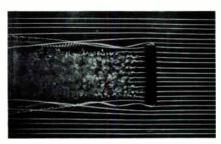
Three dimensional flow pattern on a straight wing. The formation of the wing tip vortices is demonstrated with this wing model.
