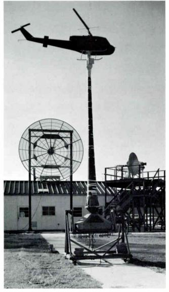
ANTENNA research range at Collins includes special support towers for holding or rotating models about one or two axes for antenna studies.
