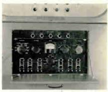
A small panel in the front door swings downward to reveal the transmitter controls. When it is lowered, the panel can he used as a desk while meter readings are being recorded. All switching and tuning controls are protected against accidental misadjustment when the panel is closed.
