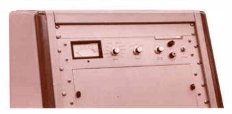
To meet the demands of the low power educational broadcaster, Collins has added a harmonic filter to the new **Phase 4** exciter to give the finest FM signal available at any price for this type of operation. The 831A-2 transmitter is completely solid state, and will provide up to 10 watts power output. Housed in an optional cabinet, or rack mounted, the 831A-2 will provide many years of trouble-free service.
