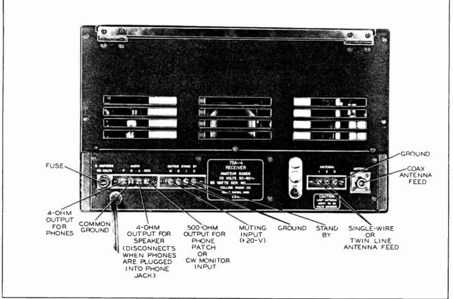
Figure 2-1. 75A-4 Receiver, External Connections
