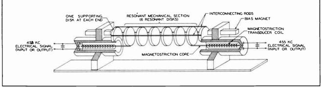
Figure 4-2. A Collins Mechanical Filter, Functional Diagram
