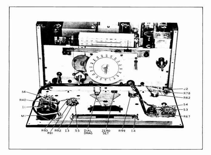
Figure 5-4. 75A-4, Front Panel Lowered
