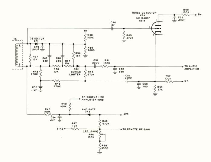
Figure 2-6. Detector, Noise Limiter, and AVC Gate, Simplified Schematic
