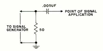
Figure 6-3. Termination to be Used in Checking 455-Kc AVC Voltage
