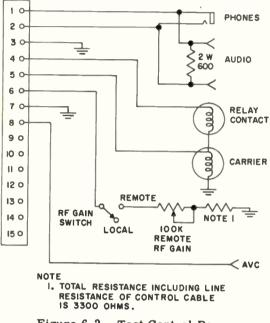
Figure 6-2. Test Control Box for 51M-8 Radio Receiver
