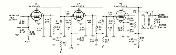
Figure 2-5. 455-Kc I-F Amplifier Circuit, Simplified Schematic
