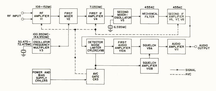
Figure 2-1. 51M-8 Radio Receiver, Simplified Block Diagram
