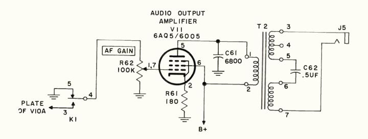
Figure 2-8. Audio Amplifier Circuit, Simplified Schematic
