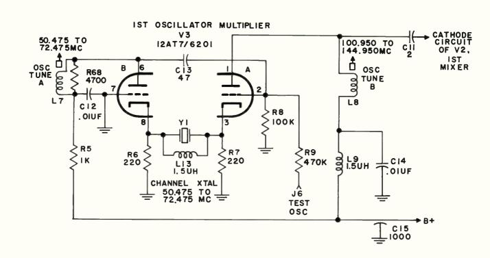
Figure 2-3. First Oscillator-Multiplier, Simplified Schematic
