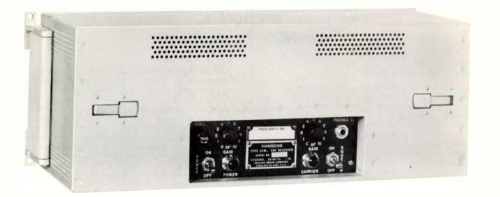
Figure 1-3. 51M-8 Radio Receiver, Showing Hinge-Type Mounting Style
