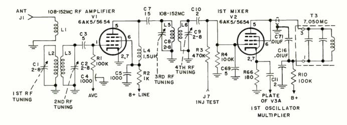
Figure 2-2. R-F Amplifier and First Mixer Circuit, Simplified Schematic
