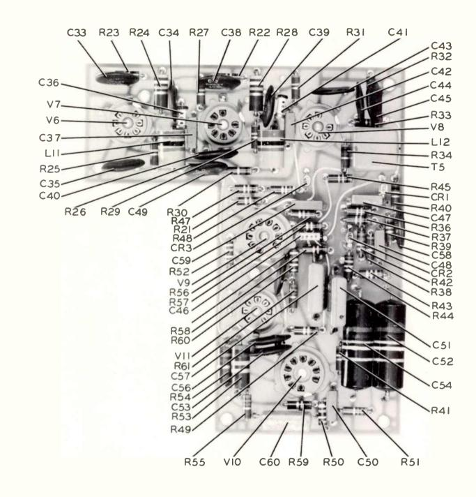
Figure 8-4. 51M-8 Radio Receiver Printed Circuit Board
