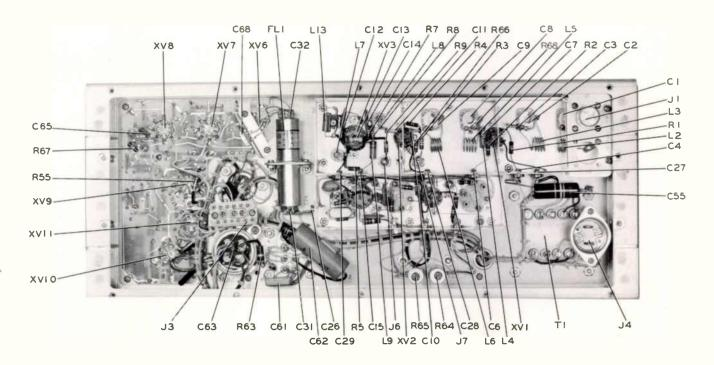
Figure 8-2. 51M-8 Radio Receiver. Bottom View
