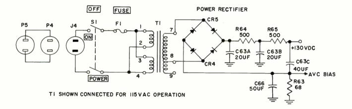
Figure 2-9. Power and Bias Supply Circuit, Simplified Schematic
