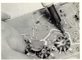
Figure 6-5. Heat-Soldered Connection on Bottom of Board
