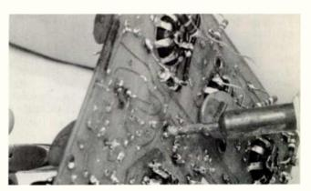
Figure 6-6. Push Leads Out Component Side of Board
