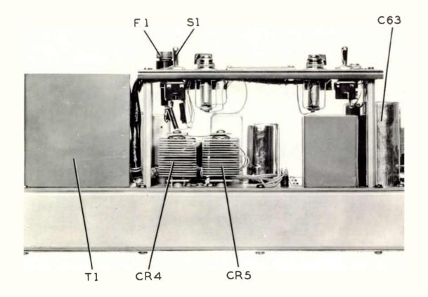
Figure 8-3. 51M-8 Radio Receiver, Power Supply Close Up
