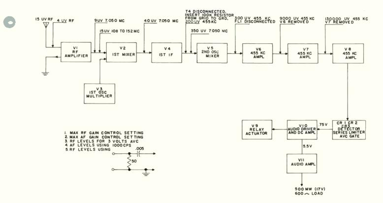
Figure 6-7. Gain Per Stage Block Diagram, 51M-8 Radio Receiver
