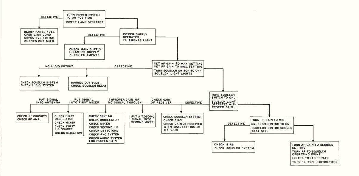
Figure 6-1. Trouble Locating Diagram, 51M-8 Radio Receiver
