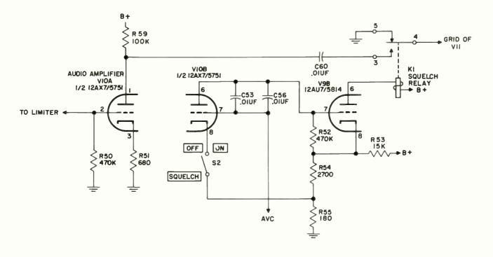
Figure 2-7. Audio Driver and Squelch Circuit, Simplified Schematic
