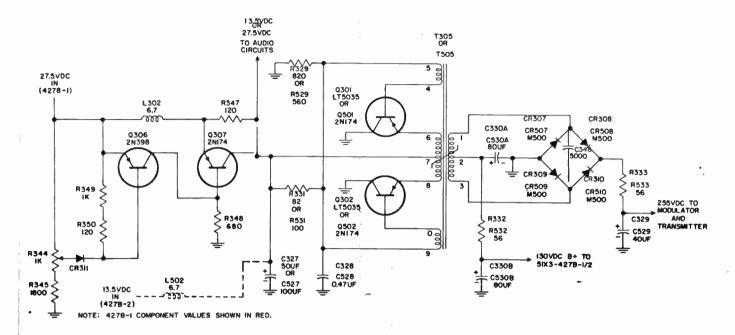
Figure 4-3. Power Supply, Schematic Diagram
