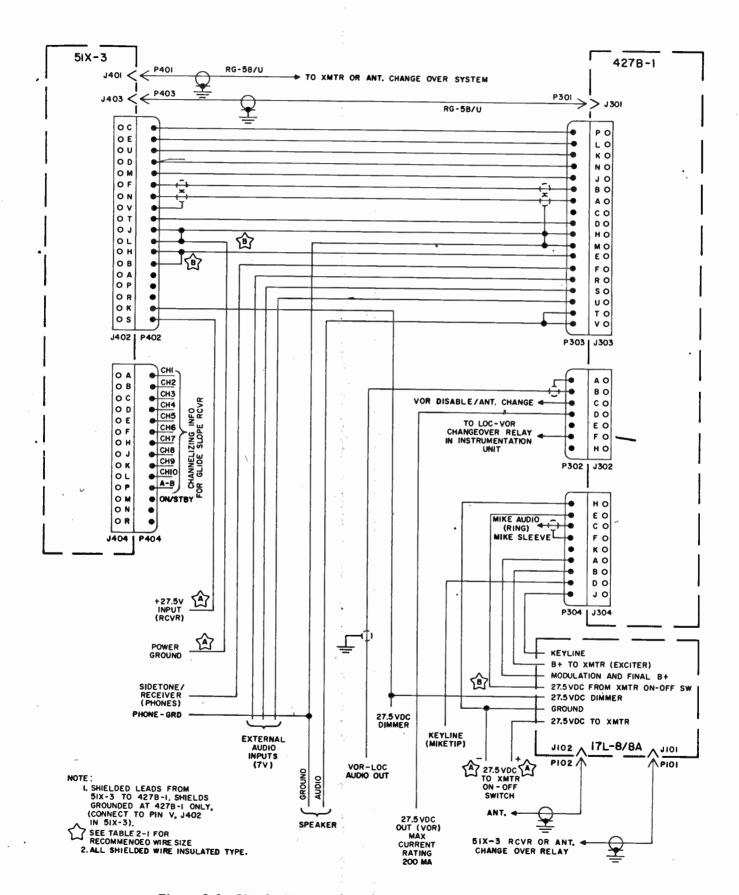
Figure 2-3. 51X-3, 427B-1, 17L-8/8A Interconnecting Cabling Diagram
