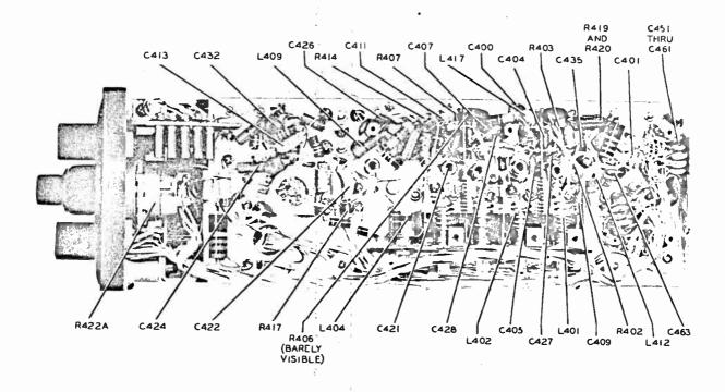
Figure 6-3A. Receiver 51X-3, Bottom View, Dust Cover and R-F Shield Removed
