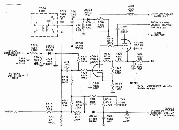
Figure 4-2. Detectors, AGC, Squelch and Noise Limiter Circuits, Schematic Diagram
