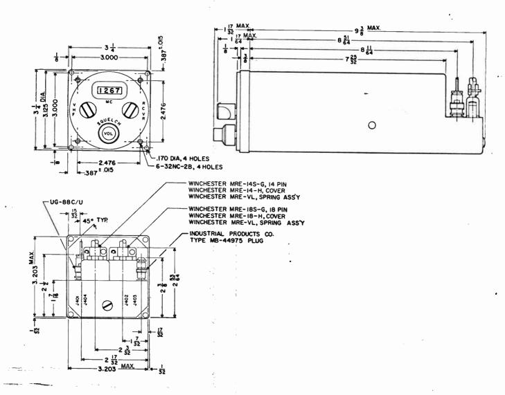
Figure 2-1. Receiver 51X-3, Installation Diagram
