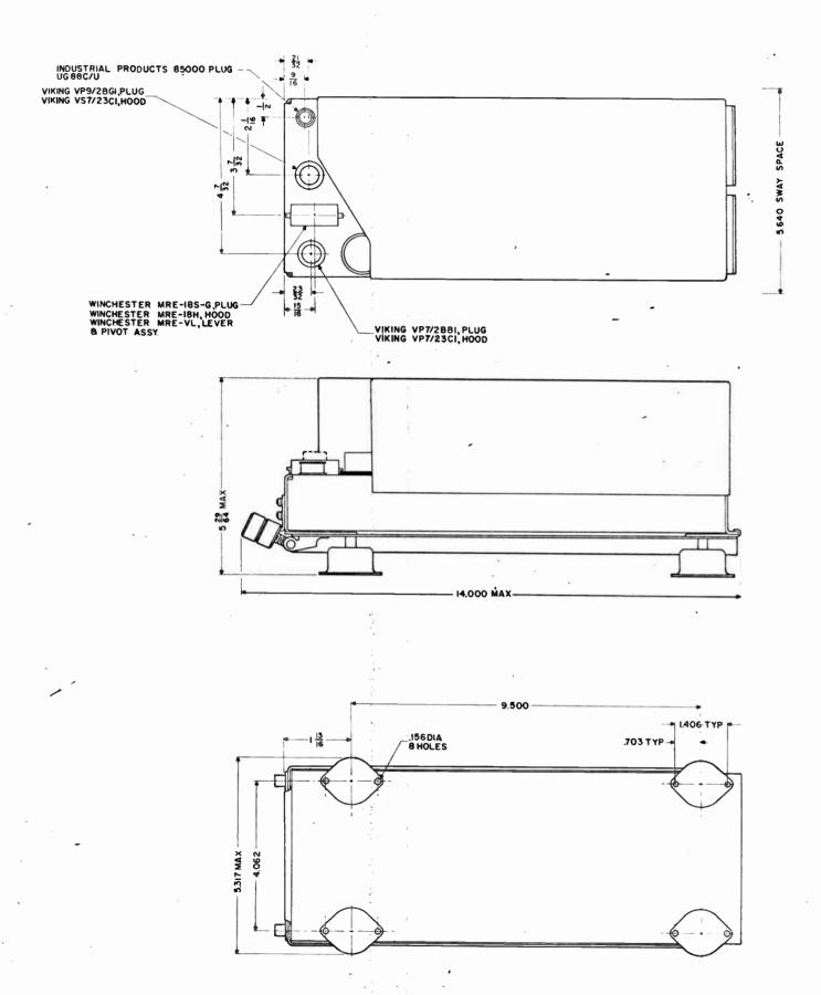
Figure 2-2. 427B-1 or 427B-2 Unit, Installation Diagram
