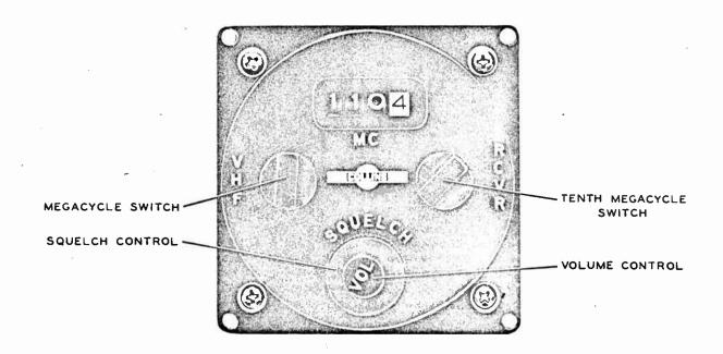
Figure 3-1. Receiver 51X-3, Operating Controls
