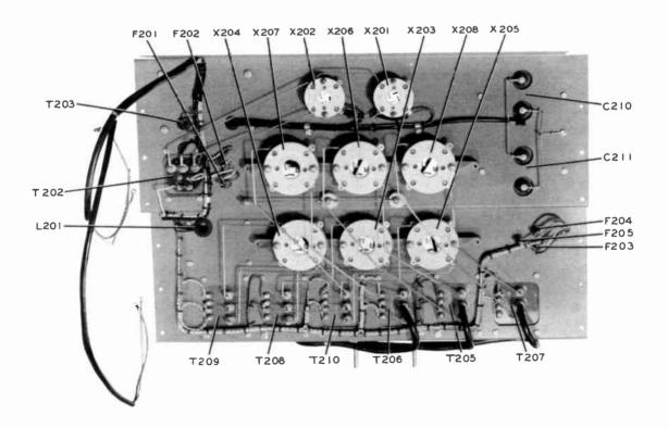
Figure 7-7. Power Supply Cabinet Rectifier Chassis, Bottom View.
