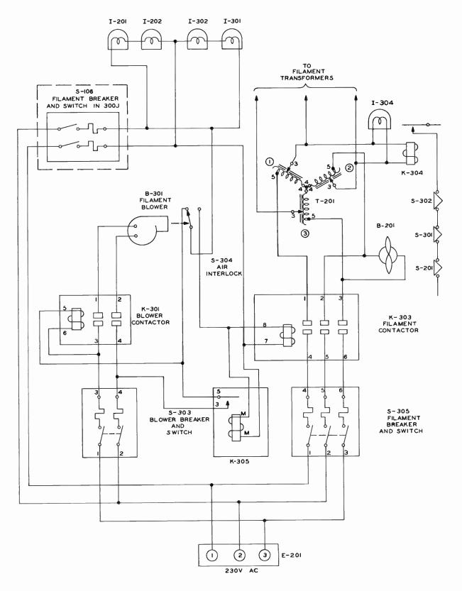
Figure 4-2. Filament Control Circuits.
