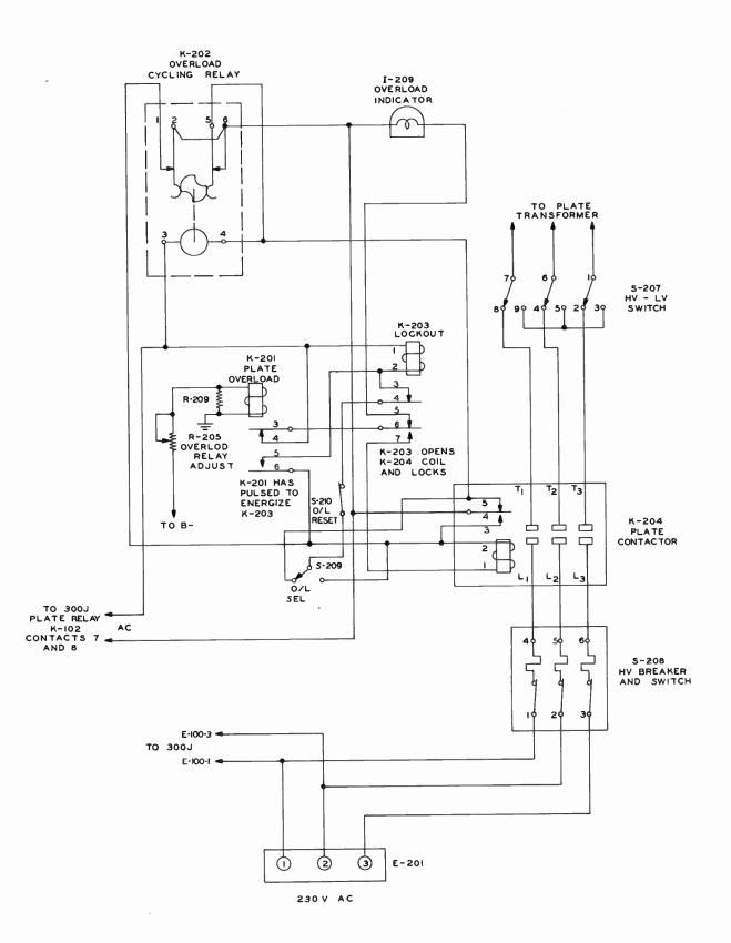
Figure 4-5. PA Plate Control Circuit, Relay Positions Shortly after Overload.
