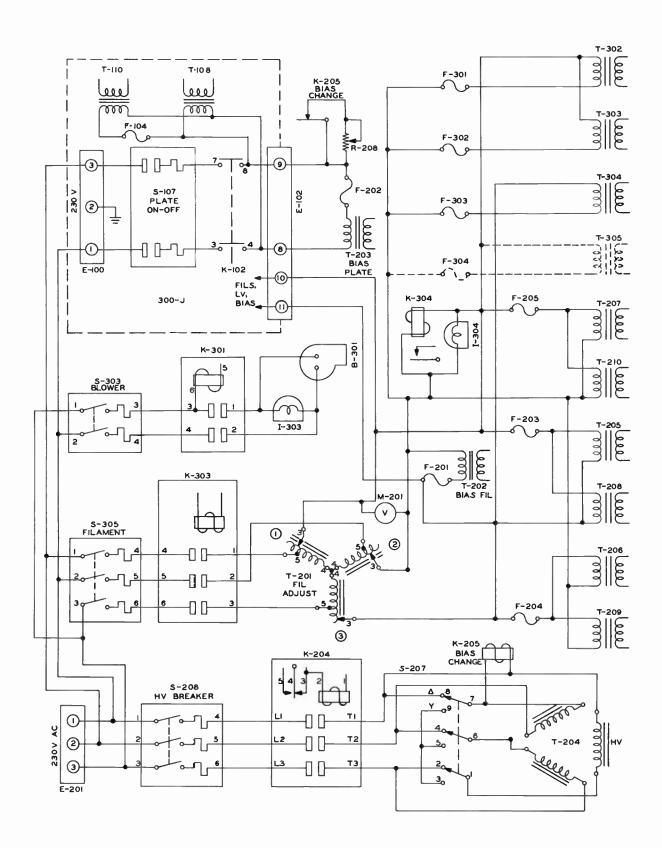
Figure 4-1. Primary Power Circuits.
