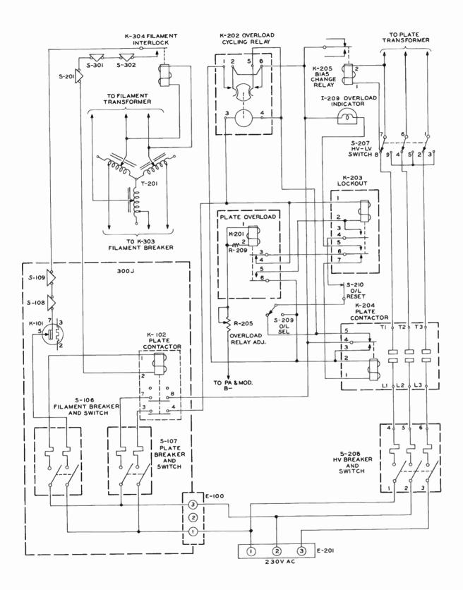
Figure 4-4. PA Plate Control Circuits -Normal.
