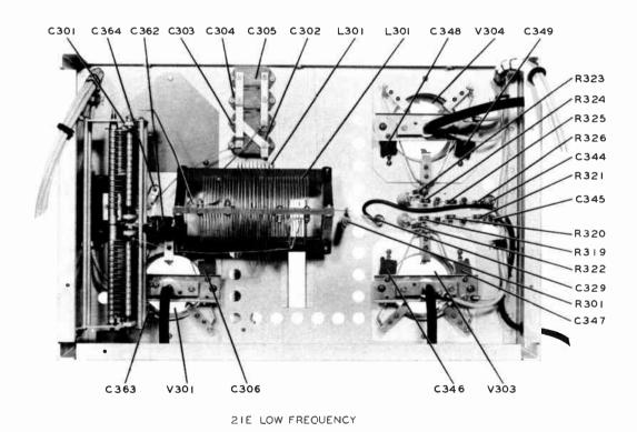
Figure 7-5A. Power Amplifier RF Chassis, Bottom View.
