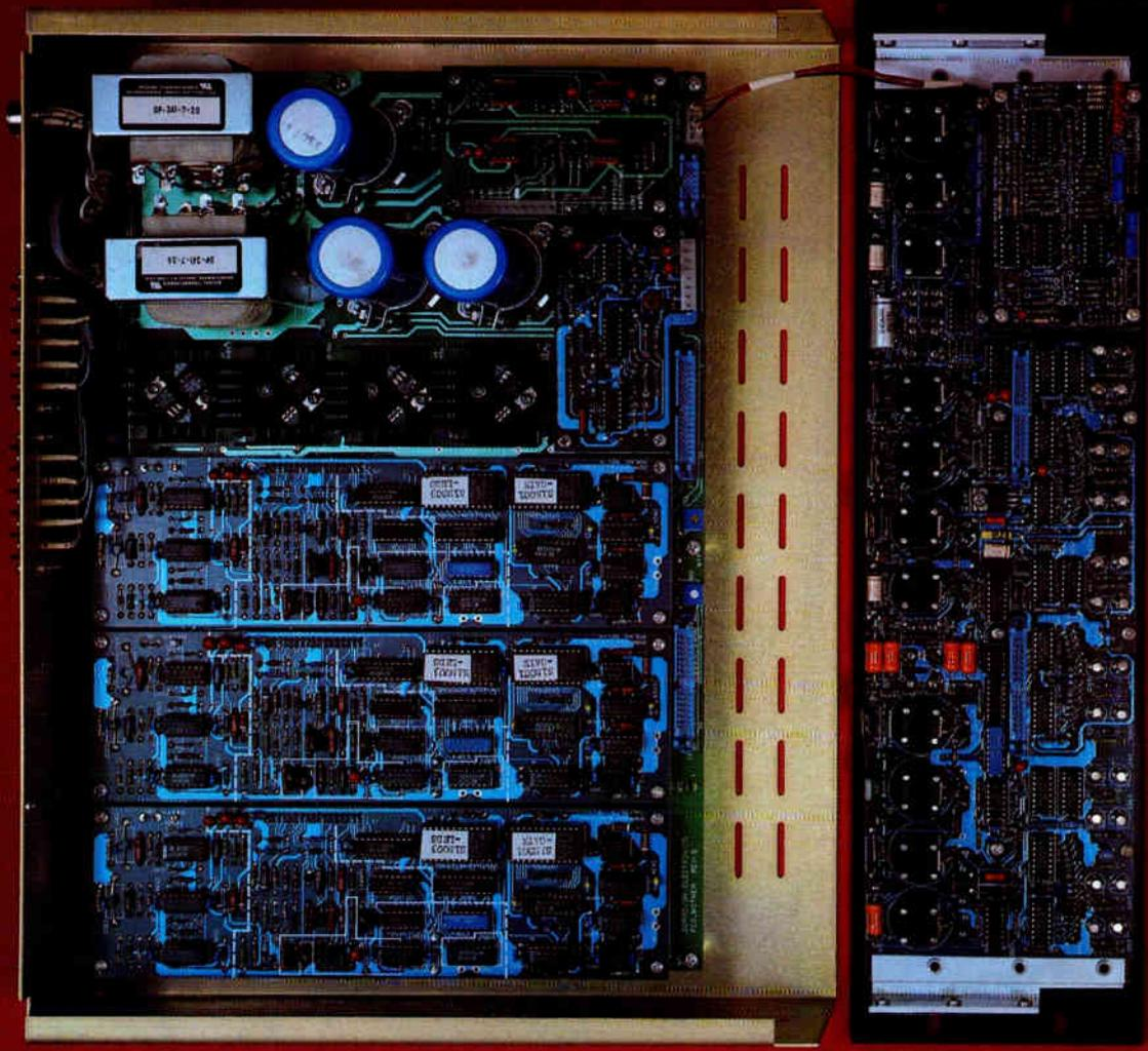
Each of the three compressor channels are powered independently and are interchangeable. The line amplifier and the peak limiter are also plug in cards. The front panel display board contains the equalizer circuit, pink noise source, and meter displays for the low, mid, and high channels.
