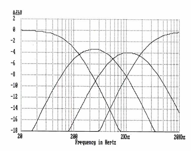
FIGURE 4-2 4 BAND FILTER RESPONSE CURVES
