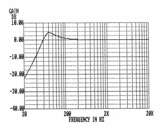
FIGURE 4-1 HIGH PASS FILTER RESPONSE CURVE
