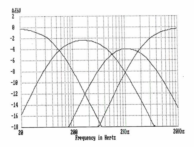
FIGURE 5-1 FOUR BAND FILTER RESPONSE CURVES (CUSTOMIZED)
