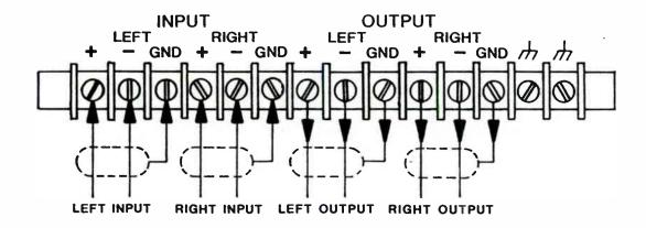
FIGURE 2-5 BALANCED LINE CONNECTIONS
