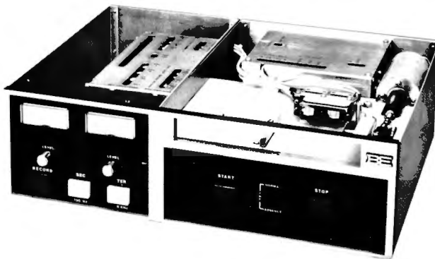
Model 4300 RPS Internal View
