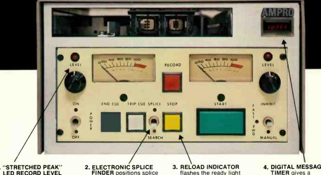
1. "STRETCHED PEAK" LED RECORD LEVEL **INDICATORS** warn of excessive record level. Standard.
