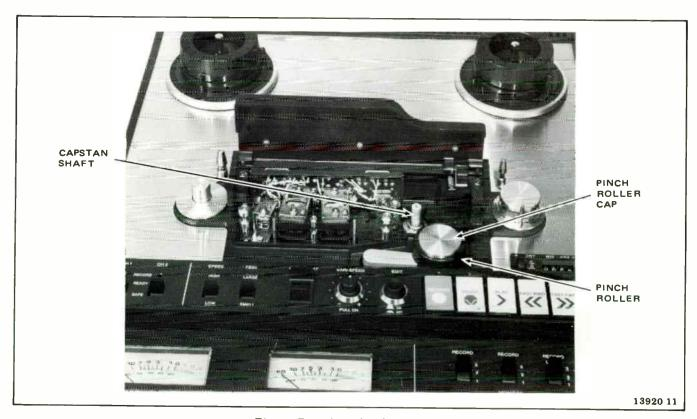
Figure 5-1. Lubrication Points
