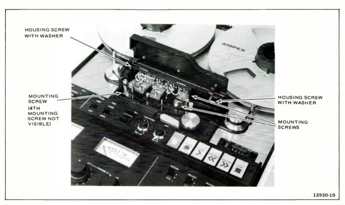
Figure 5-22. Head Assembly Removal
