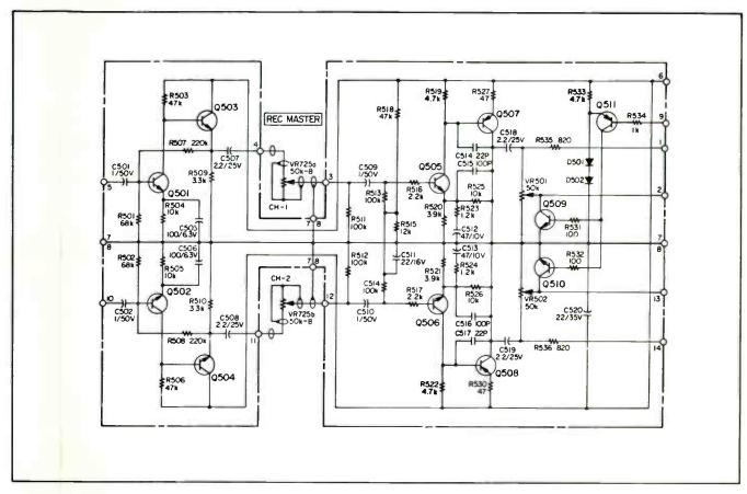
Figure 4-12. Mix Line Amplifier Schematic
