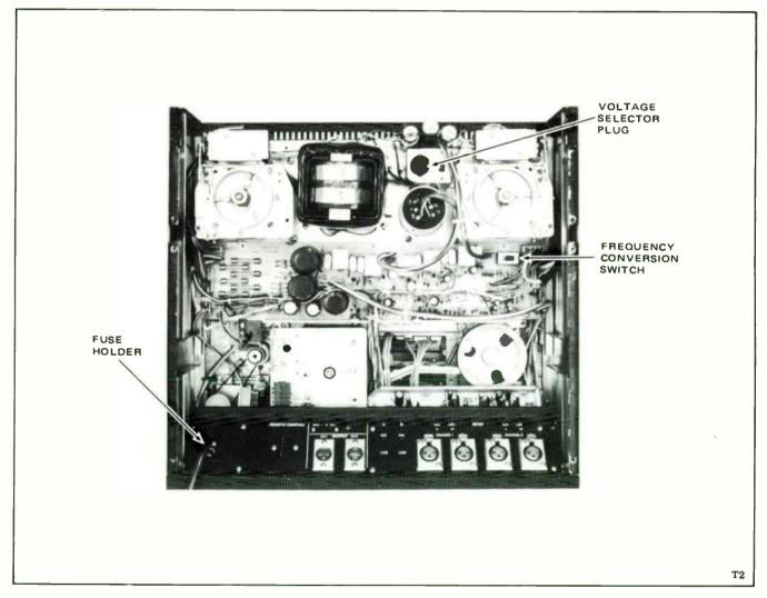
Figure 2-5. Voltage and Frequency Conversion
