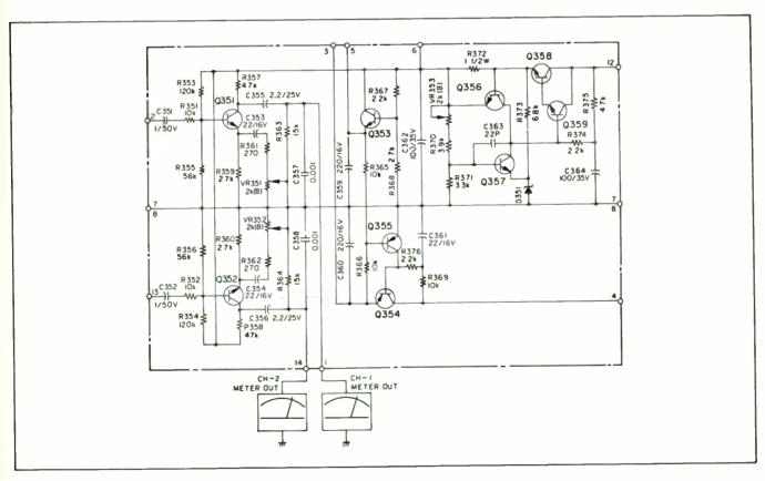
Figure 4-15. Meter Amplifier/Stabilizer Schematic
