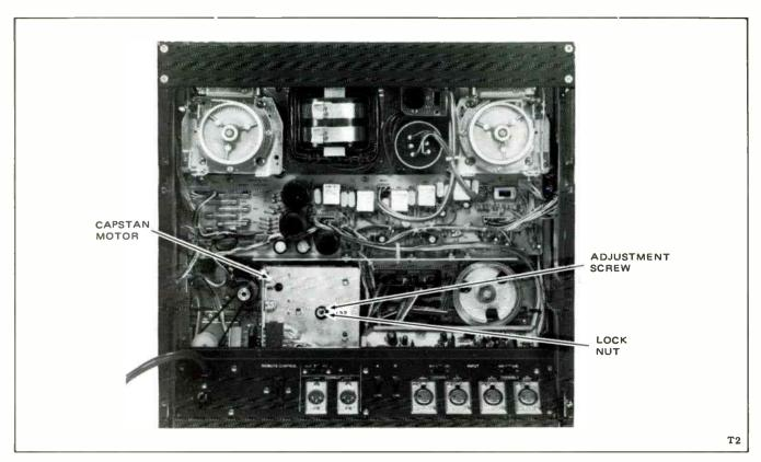
Figure 5-5. Capstan Shaft Tolerance Adjustment
