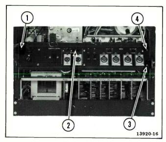
Figure 5-4. Connector Panel Screws
