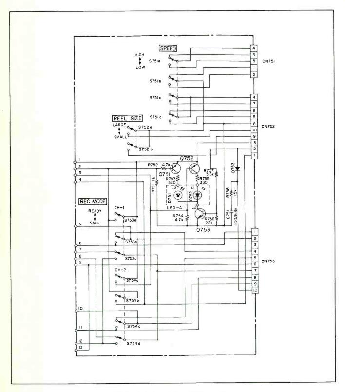
Figure 4-4. Switchboard A Schematic
