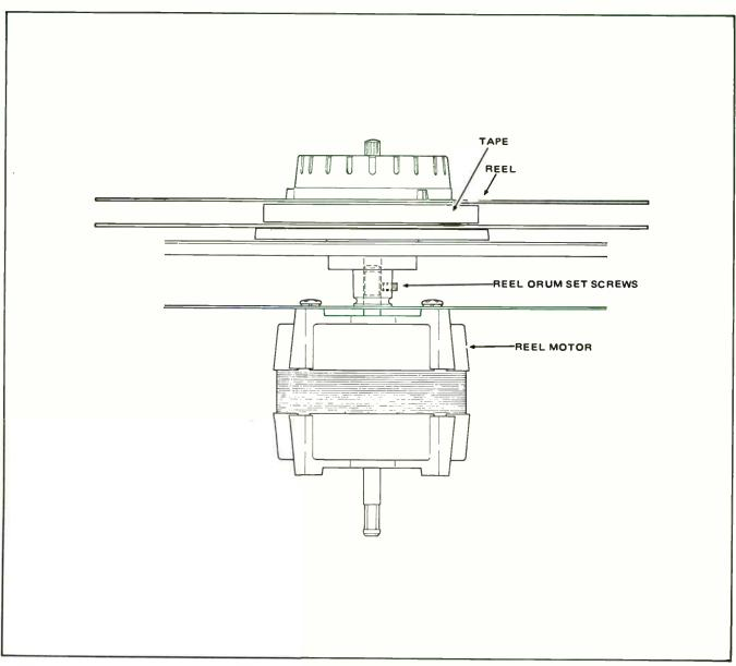
Figure 5-27. Reel Height Adjustment
