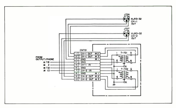
Figure 4-10. Output Transformer PWA Schematic
