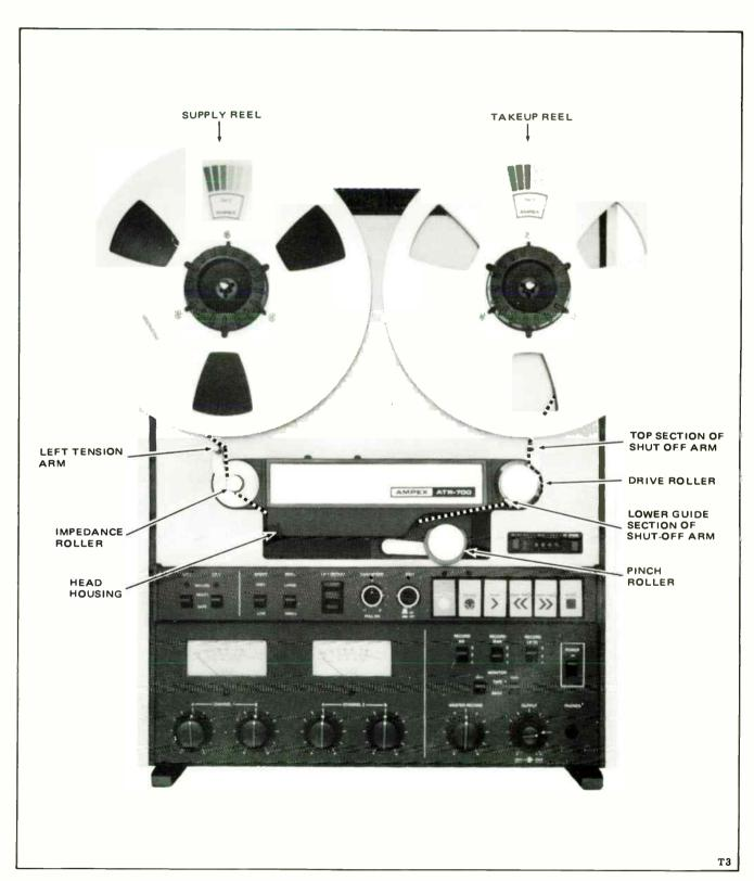
Figure 3-3. Tape Threading Path
