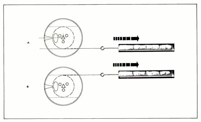
Figure 5-14. Brake Torque Measurement
