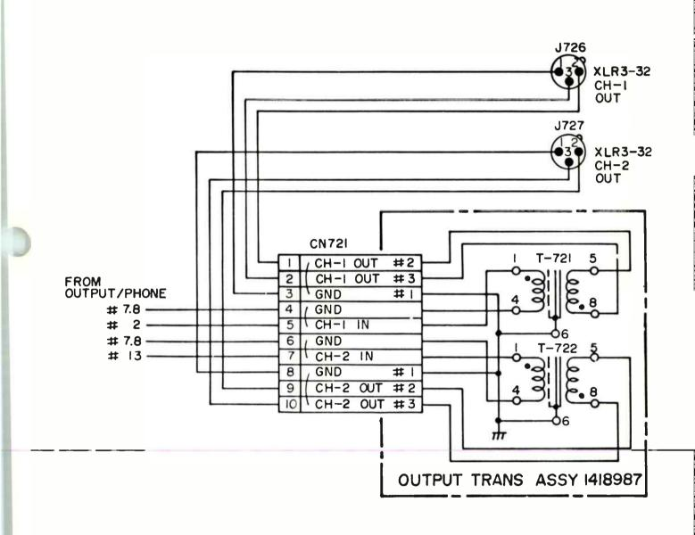
Schematic No. 1418961. Output Transformer PWA
