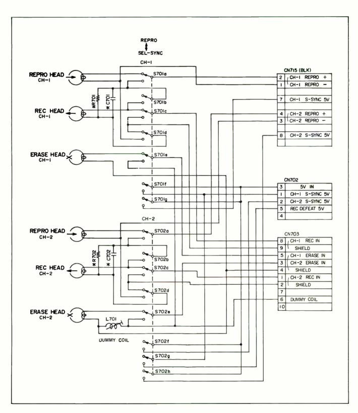
Figure 4-17. Head Assembly Schematic
