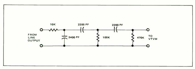
Figure 5-16. ASA "A" Weighted Filter
