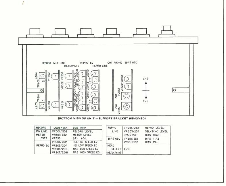
Figure 5-20. Locations of Electrical Adjustments
