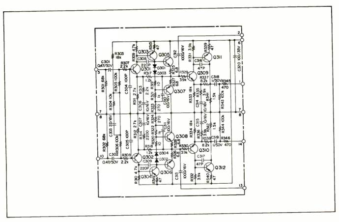
Figure 4-9. Output/Phone Amplifier Schematic
