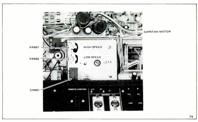
Figure 5-19. Tape Speed Adjustments
