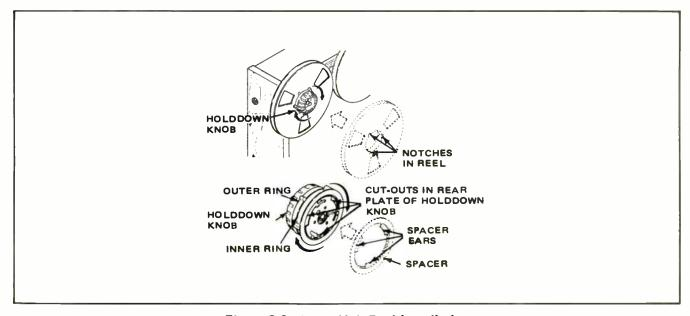
Figure 3-2. Large Hub Reel Installation
