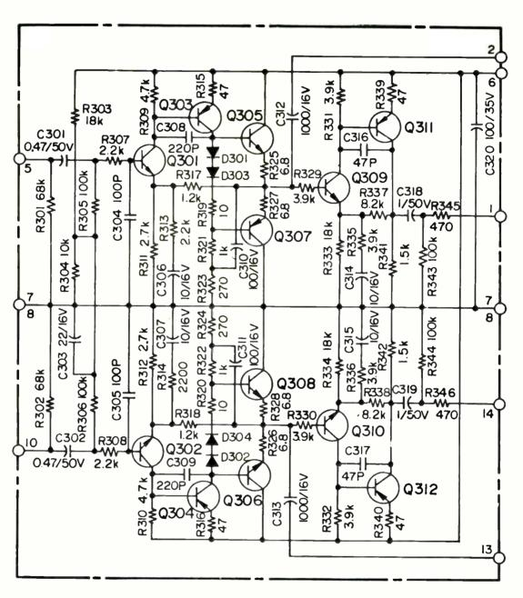
Q301,302,309,310 2SCI000 (BL,GR) Q303,304,311,312 2SA842 (BL,GR) Q305,306 2SCI567 (P,Q,R) Q307,308 2SA794 (P,Q,R) D301 ~ 304 IS2473
