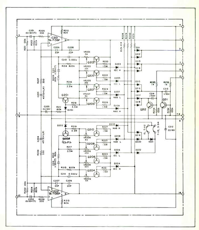
Figure 4-7. Reproduce Equalizer Amplifier Schematic
