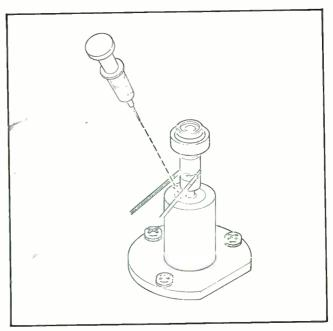
Figure 5-3. Digital Counter Roller Lubrication
