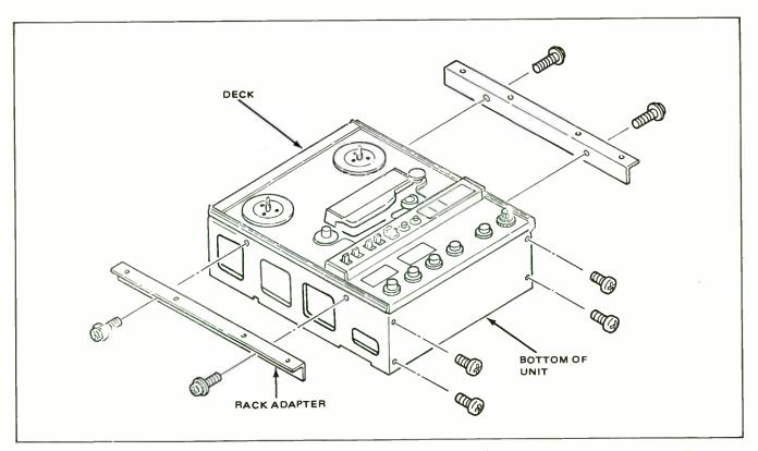
Figure 2-3. Rack Adapter Installation
