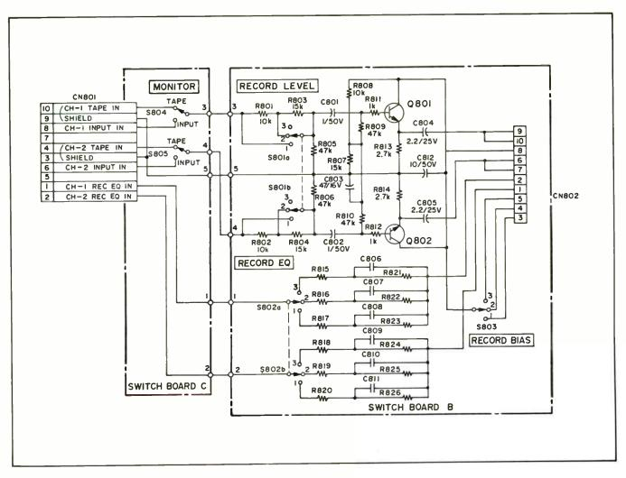
Figure 4-16. Switchboard B, C Schematic
