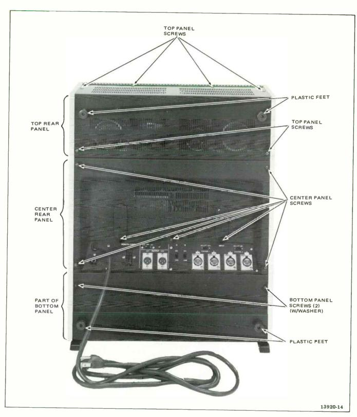
Figure 2-4. Screw Locations for Panel Removal
