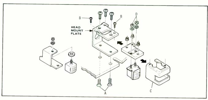
Figure 5-24. Head Disassembly
