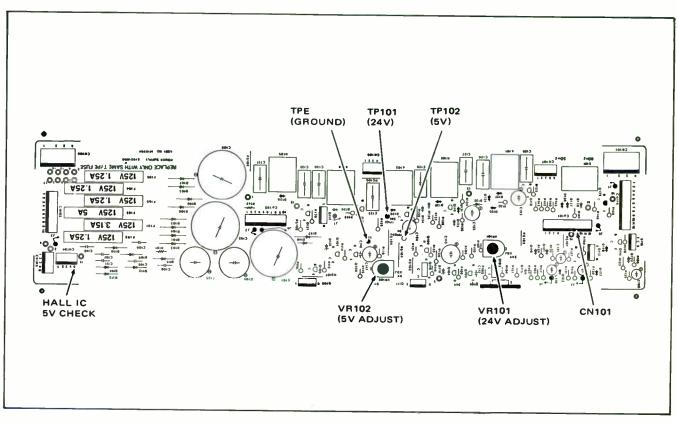
Figure 5-18. DC Voltage Adjustment, Power Supply PWA
