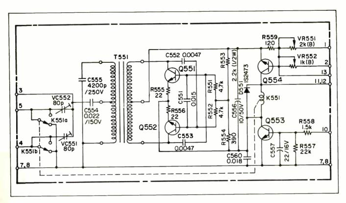
Figure 4-14. Bias Oscillator Schematic
