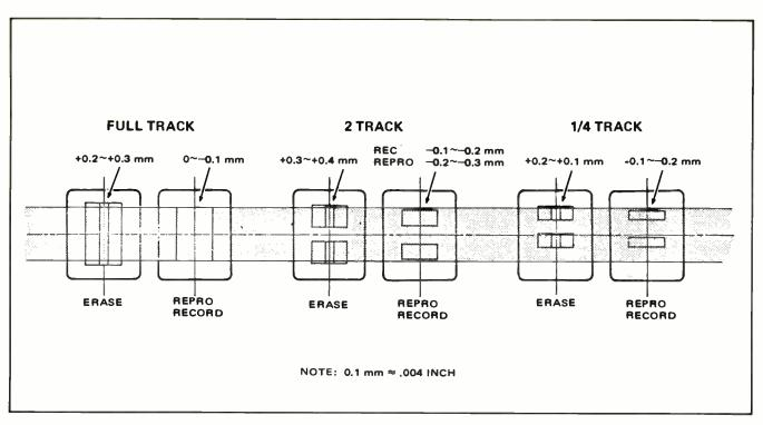
Figure 5-7. Tape Positioning for Head Alignment
