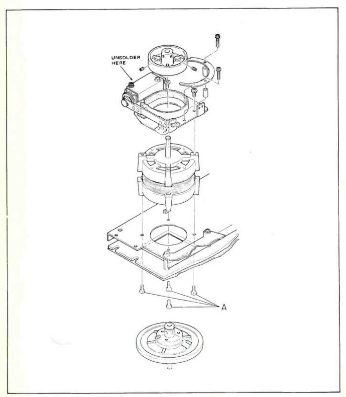
Figure 5-28. Reel Motor Assembly Removal
