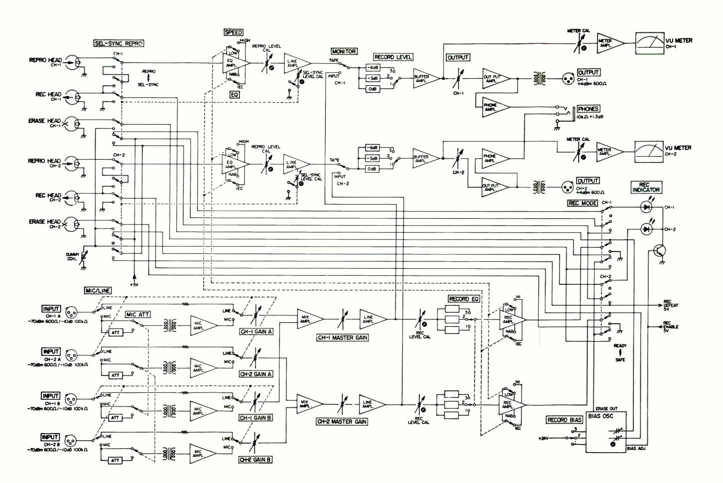
Figure 4-5. Signal System Block Diagram
