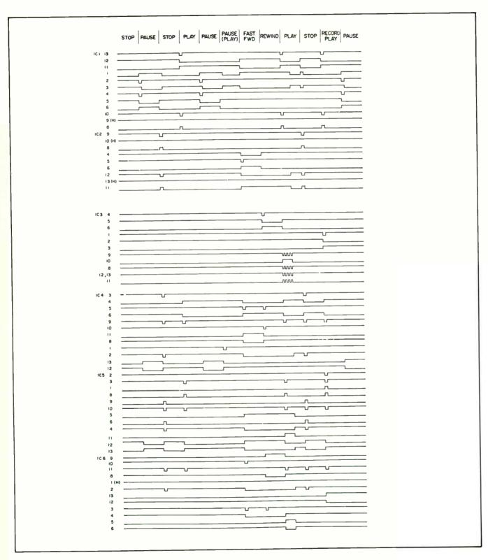
Figure 4-3. Timing Diagram (Sheet 1 of 2)
