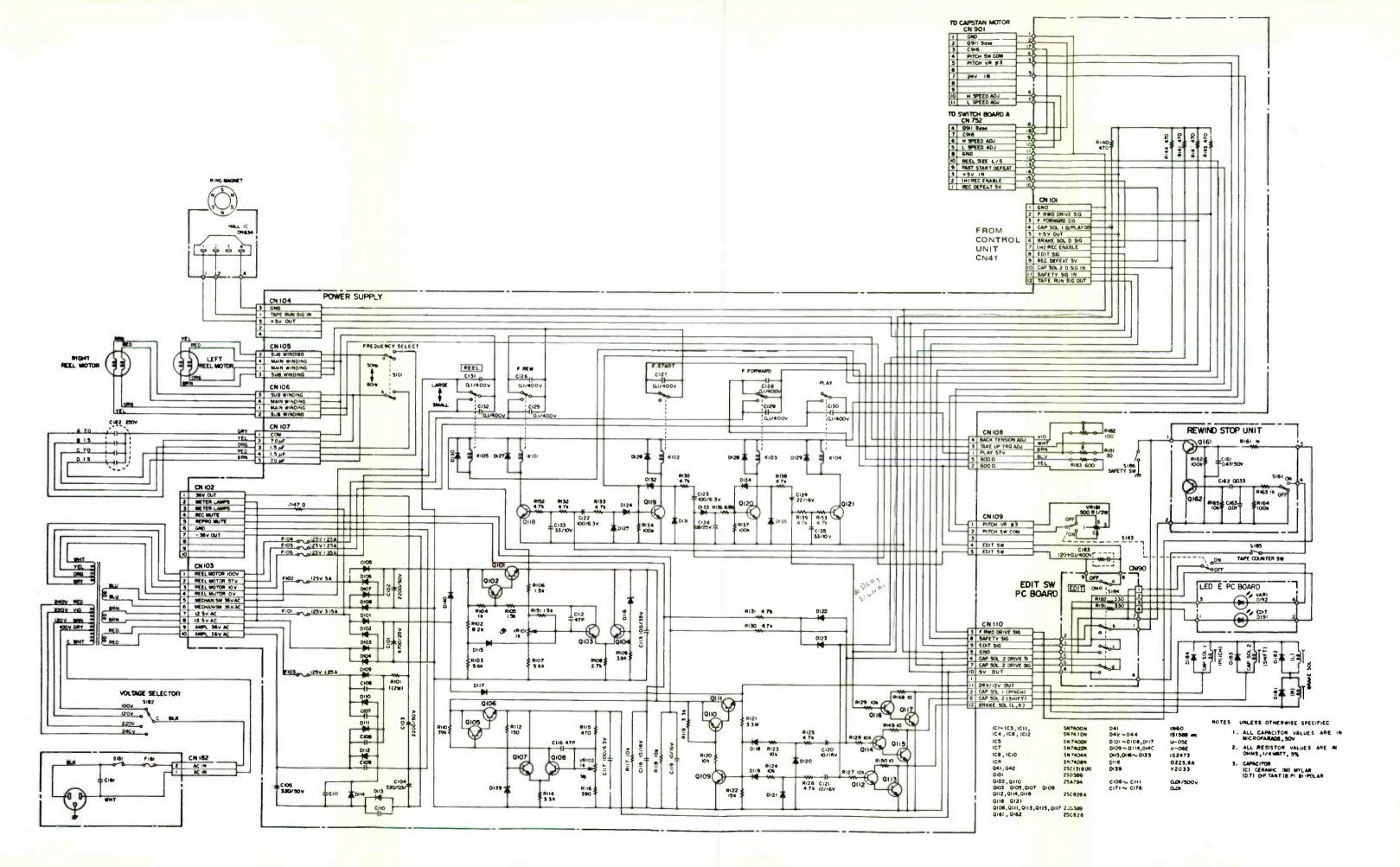
Schematic No. 1418946 Control Unit, Power Supply, Rewind Stop Unit, and Hall IC PWAs (Sheet 2 of 2)
