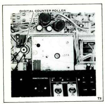
Figure 5-2. Digital Counter Roller Location
