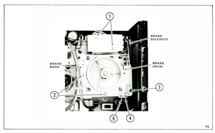
Figure 5-15. Brake Assembly
