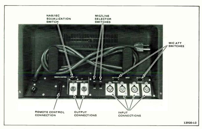
Figure 2-8. Rear Connector Panel
