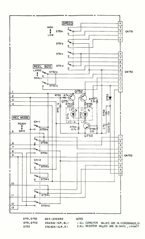
Schematic No. 1418968. Switch Board A
