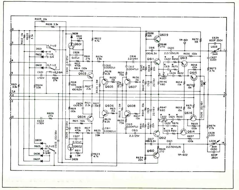
Figure 4-13. Record Amplifier Schematic
