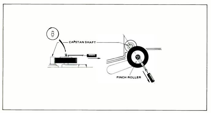
Figure 5-8. Pinch Roller Pressure Measurement
