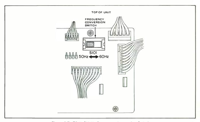
Figure 2-7. 50 Hz/60 Hz Frequency Conversion Switch
