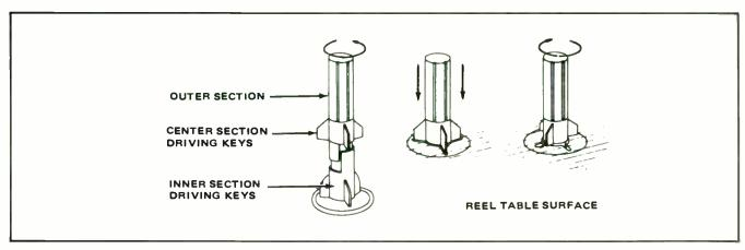
Figure 3-1. Reel Table Spindle
