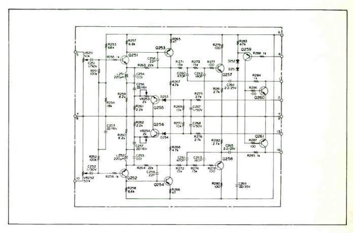
Figure 4-8. Reproduce Line Amplifier Schematic
