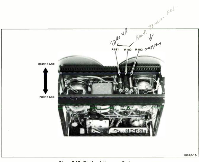
Figure 5-13. Tension Adjustment Resistors
