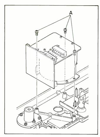
Figure 5-25. Capstan Motor Removal
