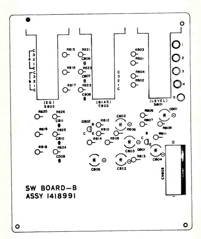
Assembly No. 1418991. Lever Switch Board PWA B
