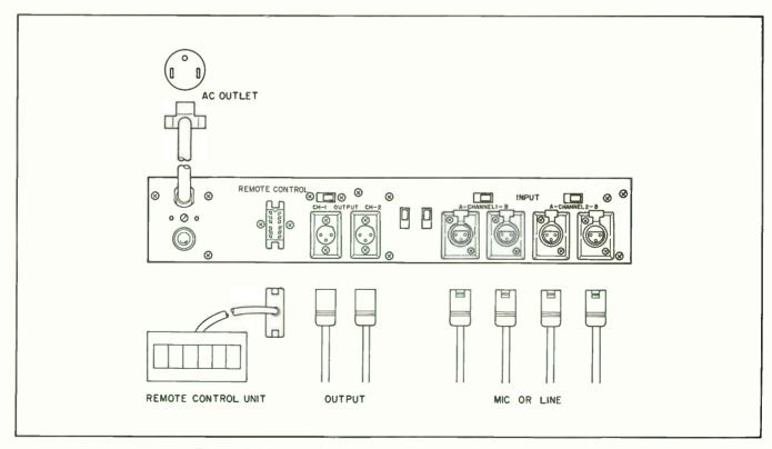
Figure 2-9. Rear Connector Panel — Initial Connections
