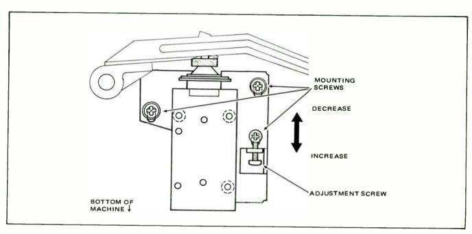
Figure 5-11. Pinch Roller Pressure Adjustment
