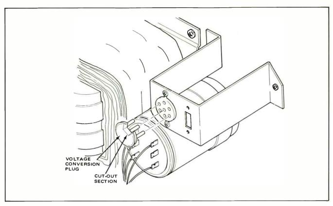
Figure 2-6. Voltage Conversion Plug
