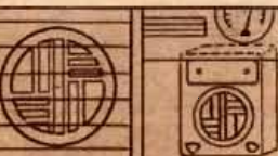
Removable speaker fits behind dash speaker grille of new cars; receiver itself mounts against car firewall.
