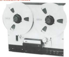
$^{1\!\!/}_{4}$ " two channel, half track reproducer with 25 Hz tone sensor, end of message and cuetone relays with adjustable delay (100 milliseconds to 15 seconds).  $7^{1}\!/_2$ -3¼ ips speeds. 19" rack mount. Designed for automated broadcast systems and other high reliability reproduce only applications. 15-7 $^{1\!\!/}_{2}$  ips speeds available on special order.
