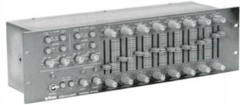
The ORBAN mono Model 672A and stereo Model 674A are cost effective, professional, quasi-parametric equalizers with the convenience of graphic type EQ controls. Wide range high and low pass filters with 12 dB/octave Butterworth slopes follow the graphic section for added versatility. Each feature has been thoughtfully chosen and cleverly implemented to make the equalizer a particularly powerful tool in nearly all areas of audio.
