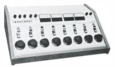
The 500SC is a rugged and versatile console designed for broadcast applications. Utilizes Allen-Bradley mod pots, VCA audio control, ITT "Schadow" switches, Electrovert screw terminal strip input and output connectors and active balanced circuitry inputs and outputs.
