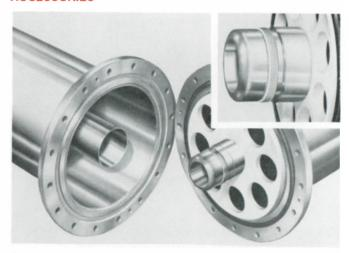
Comark rigid coaxial transmission line provides outstanding features such as constant impedance, high power capacity, and low insertion loss. Sizes to 8 3/16" Heliarc-welded flanges and wrist band bullet construction 3 1/8" and above.
