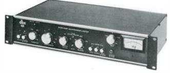
The DBX 165A is a result of combining the 165 and PEAKSTOP. The PEAKSTOP circuit which follows the compressor/limiter circuitry is a specially "soft clipper" that rounds the leading and trailing edges off the peak being clipped. By avoiding the normally sharp edges of a clipped peak, far fewer high order harmonics are generated making PEAKSTOP less audible than other types of clippers.
