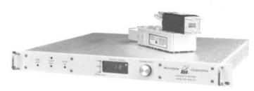
Looking for KU-Band? Allied has the most popular Microdyne 1100 BDC/DCR series! The first half of this receiver is the block down-converter (BDC) which converts the KU-Band frequencies, at the antenna, to a range of 270-770 mHz. Lower cost cable can then be utilized between the satellite antenna and the receiver. Also the BDC is available in a C-Band version which allows you to get double service from your DCR receiver!
