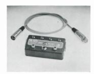
The A-10 audio accessory is a passive interface box designed to provide multiple isolated outputs from a single line-level input. Several cassette tape recorders may be driven from a single distribution amplifier line-level input. All output jacks are insulated from the case. A ground switch is provided to maximize the flexibility of the unit.
