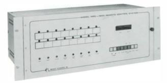
Microprocessor Remote Control System, consisting of one Control Terminal, one Remote Terminal. System is equipped with 32 command relays, 16 status channels (TTL/contact closure), and 16 digital telemetry channels. FCC acceptable for AM and FM broadcast transmitter remote control. Includes audible telco/telco data interface on each terminal.
