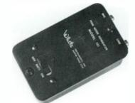
The White Instruments Model 151 is a compact, battery-powered, digitally generated pink noise generator with 268,000,000 bit word length, a flat output from 20 Hz through 20 kHz, with microphone or line level output.
