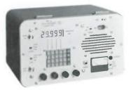
The RG-4 Receiver/Generator couples precision with reliable performance, providing an indispensible piece of test gear for broadcast engineers. An RF signal generator to excite the impedance bridge and a sensitive receiver for external null detection are housed in a single rugged case. With an OIB-1 or OIB-3, the RG-4 forms a portable impedance measuring system. Operates from 100 kHz to 29.999 mHz in 1 kHz increments. Runs off batteries, 115/230 VAC 50/60 Hz with 35 watts input power.
