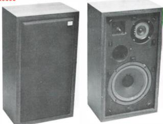
The MONITOR loudspeaker system provides a flat response from below 50 Hz to beyond 20 kHz. Its high compliance surround on the 8" woofer and phenolic tweeter combine to enhance any type of music. The tweeter control and the system fuse are behind the snap-away grille. It will handle 25 watts RMS continuous, 45 watts integrated program material at 8 ohms.
