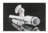
The DO-56 is a shock mounted omnidirectional dynamic microphone for hand-held broadcast applications. All handling noises and cord vibration are isolated from the microphone element. Shock isolation is enhanced by having the main acoustic cavity and the diaphragm/voice-coil assembly isolated as a unit from the case making capsule/case collision impossible.
