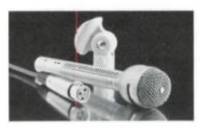
A fine, moderate cost microphone for sound reinforcement, broadcast and stage work. The RE-10 is similar in design to the RE-15, but meets requirements where somewhat more unit-to-unit variability is acceptable. It has effective directional control, little off-axis coloration, greatest rejection of unwanted sounds at 150 degrees off axis and a bass roll-off switch.
