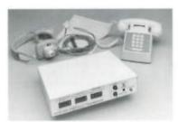
The EFT-1000 Extended Frequency Transceiver improves the sound of your telephone remotes by recovering the low frequencies normally lost on telephone lines. Audio frequencies are shifted up by 250 Hz on the transmitting end and back down on the receiving end. This preserves the low frequencies, dramatically improving the quality of the broadcast.
