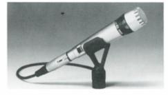
The D-1200E is a boom or hand held dynamic cardioid polar pattern microphone. Electric impedance @1,000Hz is a low 200 ohms. The three-position BMS switch permits changing response to suit individual performer and environment. Elastically suspended capsule reduces handling noise in this ruggedly constructed microphone. The SA-31 "quick-release" stand adapter is also included.
