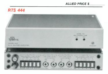
The Model 444 is a dual, two channel buffer amplifier designed to interface professional systems with semi-pro and high fidelity equipment. Although components designed for home use offer desirable features for studio applications, interconnections between the two kinds of equipment are complicated by differences in levels, impedances and balanced and unbalanced modes of operation. The 444 corrects these problems while maintaining signal integrity.
