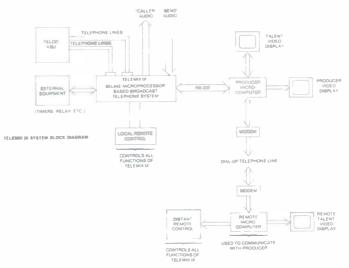
In summary, TELEMIX IX is a software driven, microprocessor based, multi-line telephone system that provides high quality telephone audio. The sytem is software driven, allowing maximum flexibility in processing telephone lines. The RS-232 port permits long distance remotability and in-house programming via a minicomputer. The system uses an advanced design telephone hybrid that produces produces clean, clear audio.
