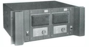
As opposed to the "fix-it-up-with-feedback" approach in common use today, UREI carefully departed from conventional design techniques. Each amplifier stage in the 6500 was engineered for optimum performance with no overall feedback. The 6500 features two channels on an independent, modular plug-in chassis with front panel access. The 6500 is rated at 275 watts into 8 ohms per channel output with .1 THD.
