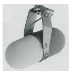
Specifically designed to minimize boom microphone problems in television studio and location applications, the SM-5B is also excellent for radio deejay use. A smooth, wide-range frequency response with moderate presence rise makes it especially suitable for vocal pickup as well as scoring assignments. The SM-5B has a cardioid pickup pattern with exemplary off-axis uniformity, even at
