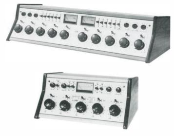
The LPB SIGNATURE II consoles feature transformer audio inputs. Monitor speaker muting and on-air light relays are provided. A cue position is provided in each mixer and all models include an internal cue system consisting of a cue amplifier, level control and 5 speaker. The internal monitor amplifier is switch selectable to monitor program or two external monitor inputs. The illuminated VU meter reads the program output at all times.
