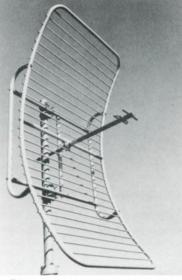
The Scala PR-450-U<sup>™</sup> is widely used in point to point communications and telemetry systems in the 350 to 1000 mHz spectrum. Paraflector<sup>™</sup> performance approximates that of a parabolic dish of the same aperture, and is easier to assemble and install. The PR-450U offers rugged construction for reliable long-term service, even in severe environmental conditions.
