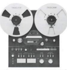
A half-track ¼" master recorder/reproducer with 10½" reel capacity, 15-7½ ips speeds, independent L & R record mode, simul-sync, full frequency response in sync mode, function and output select and punch in/out recording. The 32 also features  $\pm$  12% pitch control, dump edit, mic inputs, independent input/output level controls, headphone jack with volume control, cue control, FL tape counter and zero return.
