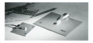
The pressure recording process, invented by Long and Wickersham, introduced a bright new concept to audio engineering. They discovered that sound approaching a boundary such as a floor, wall, table, podium, etc. creates a thin zone in which the direct and reflected signals are coherently in phase and reinforce each other. The Crown PZM microphone creatively realizes the potentials of that invention offering significant improvements in signal clarity and range. Comb filtering is eliminated.
