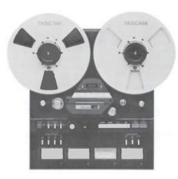
A 4-track  $\frac{1}{2}$ " recorder/reproducer with 15-7½ ips speeds,  $10\frac{1}{2}$ " reel capacity, full frequency response in sync mode, function and output select and punch in/out recording. The 34 also features  $\pm 12\%$  pitch control, dump edit, cue control, FL tape counter and zero return.
