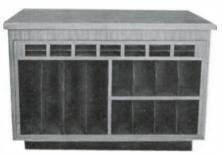
A-LINE turntable bases are constructed of %'' high-density particle board covered with standard laminates. Tops are 1%'' thick. Turntable bases are normally supplied with rack rails constructed of 11 gauge steel, tapped to accept 10-32 standard EIA rack panel screws. Cover panels are available at \$6 per bay. Custom cabinets with record and/or tape storage inserts are available.
