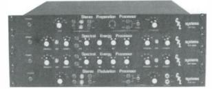
This is the ultimate FM system. Maximum fidelity, maximum loudness and maximum control. The FM-4 connects to your stereo generator and includes SPP800, a PREPARATION PROCESSOR, a two band AGC that is gated to prevent noise pull up, SMP800, an FM STEREO MODULATOR PROCESSOR, that provides absolute peak control and maximum fidelity and one SEP800 SPECTRAL ENERGY PROCESSOR, four band compressor/expanders with gating in each band.
