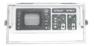
The Crown RTA-2 is designed for audio-range real-time spectrum analysis in 1/3 and full octave bands. All the sub-systems needed to perform quick, accurate on-site equalization of sound-reinforcement systems are included in the RTA-2.
