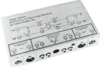
The HH 2 x 2 level matching interface is a line amplifier/attenuator which interfaces +4 or +8 dBm professional recording or broadcasting equipment with -10 dBm high fidelity and semi-pro equipment. Because the unit is transformerless, it achieves improved transient response. Each HH 2 x 2 level matching interface is a complete stereo system. Indeed, it is a stereo amplifier which boosts -10 dBm signals to a nominal +4 or +8 line level output.
