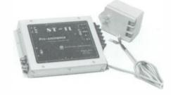
The ST-11 Pro-eminence phono pre-amp by Micro-Track is a super high performance unit. It is RFI resistant for use in AM, FM or TV. It is very compact and designed to match a 47K ohm magnetic stereo phono cartridge. Provision for a nominal 0 dBm output with headroom to a max. of +22 dBm. Distortion is .05 or less, THD and IM. The signal to noise ratio is -72 dB or better, also has a jumper selectable rumble filter internally.
