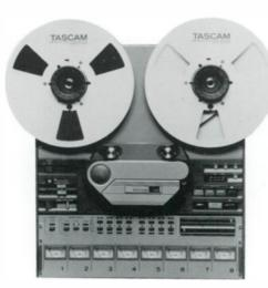
An 8-track  $\frac{1}{2}$ " 8 channel production recorder/reproducer with -10 RCA input/output,  $10\frac{1}{2}$ " reel capacity, full frequency response in sync mode, full servo, SMPTE interlock capability through an accessory connector and punch in/out recording. The 58 also features pitch control (15% coarse/0.7% fine), manual tach wheel edit, dump edit, search to zero and search to cue and 15 ips speed.
