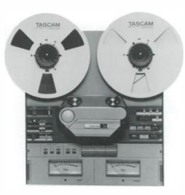
A 2-track ¼'' 2 channel half track mastering and broadcasting recorder/reproducer with +4 XLR/-10 RCA input/output, 10½'' reel capacity, sync capability, full servo and SMPTE interlock capability through an accessory connector. The 52 also features punch in/out recording, pitch control (15% coarse/0.7% fine), manual tach wheel edit, dump edit, search to zero and search to cue and 7½-15 ips speeds.
