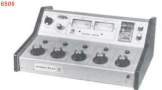
The Model 6509 audio console features five mixing channels, nine mixing inputs, outputs for stereo, mono, monitor, headsets and cue speaker, selectable muting, slotted screw terminal connections, illuminated VU meters. Crosstalk spec'd at -50 dB to -74 dB and distortion is 0.4% Re: +8 dBm output, 800 Hz, hi level input. Package size is 1734 W x 1234 D x 612 H and weighs 16 lbs.
