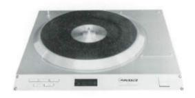
The new RUSSCO direct drive turntable is equipped with a unique magnetic induction braking system which disengages automatically after bringing the platter to a stop. Speed controls use quartz synthesized PLL techniques. All controls are on a slanting front panel within view of the operator.
