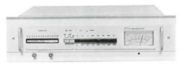
The heart of any Broadcast Electronics FM Transmitter is the FX-30 synthesized exciter.
