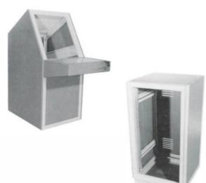
The DR series of H.O.M.E. 19" modular racks includes several features including sturdy welded construction of 16 gauge CRS, optional side panels that are removable for multiple bolt-together assemblies, adjustable 11 gauge angles tapped for 10-32 screws on standard EIA spacing that makes panel mounting easy. A cable opening is provided in the bottom panel. A rear door with lock and handle is provided. You can choose from 20 standard baked enamel colors. Depths to 24" available.
