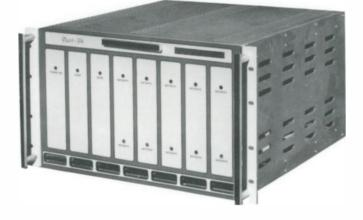
For Digital Satellite reception we recommend the FAIRCHILD DART 384 (formerly known as the COMTECH DART 384). The DART 384 receiver consists of down-converter, receiver-demodulator shelf, audio program channels, voice cue channels, and data program channels.
