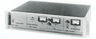
The SM2200 Stereo Generator consists of a sub-carrier oscillator, balanced modulator and channel amplifier, packaged in a modular unit for use with the FMX-2200S.
