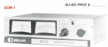
The SCM-1 SCA Frequency and Modulation Monitor, when added to the FMM-1 provides complete monitoring and test functions for SCA storecasting and remote telemetering applications. Up to four crystal switch positions allow four channels to be operated and tested.
