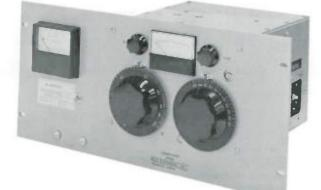
The Common Point Impedance Bridge is an invaluable device for directional array maintenance. The CPB-1 is designed for permanent installation in existing phasing equipment to provide an accurate indication of the common point impedance. The CPB-1 will handle common point powers of up to 5 kW with 100% modulation. The CPB-1A is designed for powers up to 50 kW.
