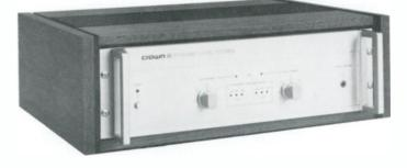
The CROWN Power Line Three is a rack-mounted power amplifier rated at 90 watts per channel into 8 ohms, with a T.H.D. of less than .05%, and I.M.D. of less than .05% and a slew rate of 12 volts per microsecond. The frequency analyzing display shows peak levels in all three frequency bands, provides information on spectral balance to check system, music, amplifier, speakers or room.
