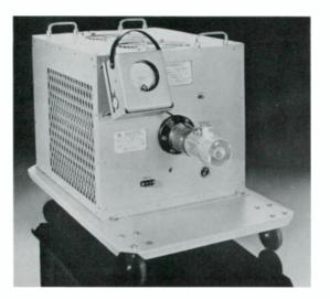
\* Power rating 25 kW continuous duty up to 900 mHz
