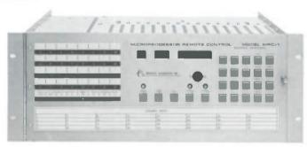
Microprocessor Remote Control System. Includes one Control Terminal and one Remote Terminal. Up to nine Remote Terminals function with a single Control Terminal. For 2-wire or 4-wire dedicated wireline or equivalent interconnecting circuits. Basic system equipped for 16 command lines (open collector electronic switching), 16 status channels (TTL/contact closure), and 16 telemetry channels indicated as 16/16/16. OPTIONS PRICES UPON APPLICATION.
