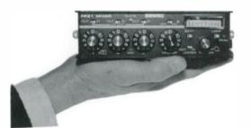
The Model FP-31 is a compact, portable microphone mixer specially designed for electronic news gathering (ENG) and electronic field production (EFP) use including film, video and remote broadcast applications. The FP-31 provides a wide, flat frequency response, low distortion, and up to +18 dBm output. The unit features extremely low internal noise and switchable low-cut filters for each input that effectively reject low-frequency handling and wind noise. 400 Hz slate tone, 1 kHz cue tone.
