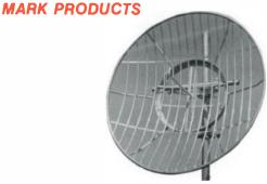
Mark Products offers a variety of sizes of Heli-Arc welded aluminum Multi-element Grid Parabolas for point to point relay operation in the 400 to 2700 mHz frequency range. The patented grid of construction is lightweight, yet extremely strong. One of the outstanding advantages of the grid antenna is that it has wind loading characteristics of only 25 to 40% of comparable size solid parabolas.
