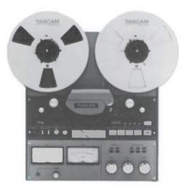
A 2-track '4'' 2 channel half track mastering and broadcasting recorder/reproducer with  $10^{1/2}$ '' reel capacity, sync capability, full servo, SMPTE interlock capability through accessory connector and punch in/out recording. The 42 also features NAB or IEC equalization, dump edit, search to zero and search to cue,  $7^{1/2}$ -15 ips speeds and +4/-10 input/output.
