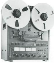
$^{\prime\prime}$  '' four channel, quarter track recorder/reproducer. DC-servo capstan with  $\pm$  7% vari-speed. 15-7½ ips speed. +4 or -10 dB input/output level select. Real time tape counter with LED display. Zero return. Headphone output with channel select. Test oscillator (1kHz or 10 kHz). Microprocessor controlled transport logic. Dynamic braking. Integral splicing block. External machine control interface connector for synchronizers.
