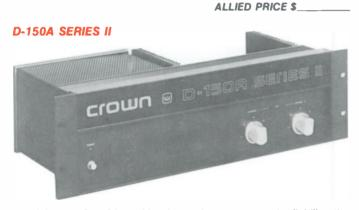
Retaining the D-150A tradition for sonic accuracy and reliability, the CROWN D-150A Series II is rated at 80 watts per channel into 8 ohms, 250 watts into 8 ohms mono. The frequency response is  $\pm 0.1$  dB DC to 20 kHz at one watt into 8 ohms;  $\pm 1$  dB DC to 100 kHz., less than .001% harmonic distortion, less than .01 I.M. distortion and 6 volts per microsecond slew rate.
