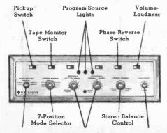
5-Position Input Selector Bass and Treble Controls For Each Channel
