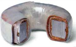
The Delta Series incorporates a new innovation in domestically made cartridge machines, the toroidal power transformer, distinguishable by its doughnut shape. The magnetic core is made of spirally wound magnetic steel, and the primaries and secondaries are wound through the center and
