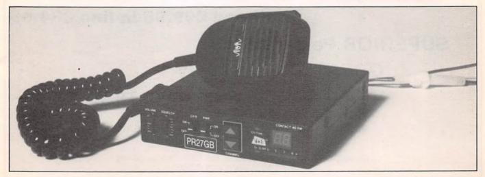
The only other point is that the volume and squelch controls are a little fiddly to operate, particularly whilst mobile over less than perfect roads. The short travel makes fine adjustment awkward and although somewhat a matter of personal preference, I feel two conventional rotary controls here would be a lot better
