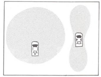
Boot mounts give a wide spread with less signal behind you. While Co-phased antennas give a forward and back signal, providing they are far enough apart.
