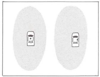
A roof mounted antenna throws a good signal forward and backwards, in an equal pattern. The gutter mount is not so equal.
