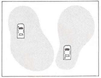
A wing mount throws the signal over your shoulder and diagonally opposite, or forward at an angle if mounted on the rear wing.
