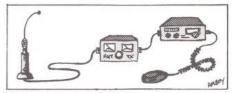
The SWR meter should be connected between the antenna and the rig using a short patch cable.
