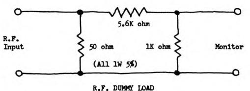
Build above circuit in Aluminum Mini-box for shielding.
