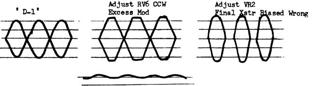
Undermodulation Adjust RV6 CW
