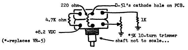
To align the frequency, center up the knobs and adjust all three modes for center slot. Now, decide how much slide you will need. The slide is adjustable from 5KHz to 20KHz, but only in the down portion. Upwards amount of slide will remain the same. Reason: Voltage is remaing constant at the top of control; but can adjust resistance to ground with the 10-turn trimmer; thus can control the amount of voltage drop. In most cases the slide up will be about 7KHz and down about 13KHz.
