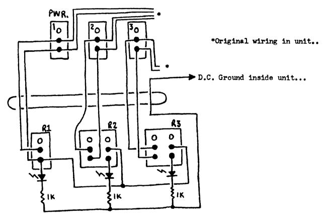
Note: Switch R1; this does not have an added section; isn't needed for the main power switch. R2 and R3 do have the added section for indication lamp circuit.
