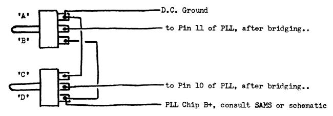
Both sw's in OFF position, normal 40 ch. operation ..
