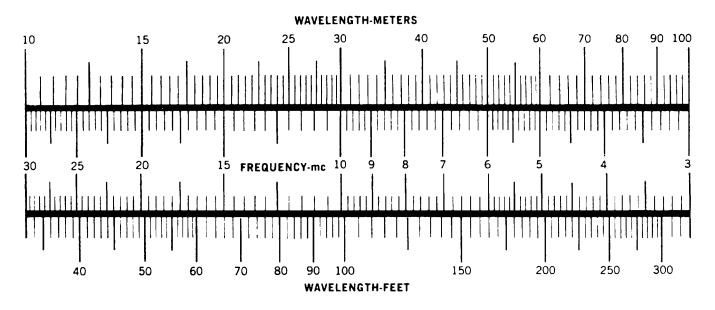
Wavelength-frequency conversion may be quickly made with chart above. Usefulness of chart is readily extended by using powers of 10 on coordinates. Example: Fø scale (MHz) is multiplied by 10<sup>3</sup> (for GHz), multiply wavelength scale (feet and meters) by the reciprocal of 10-3 (for millimeters). For Calculation: meters= 300,000/fKHz= 300/fMHz, or ft= 984,000/fKHz = 984/fMHz.
