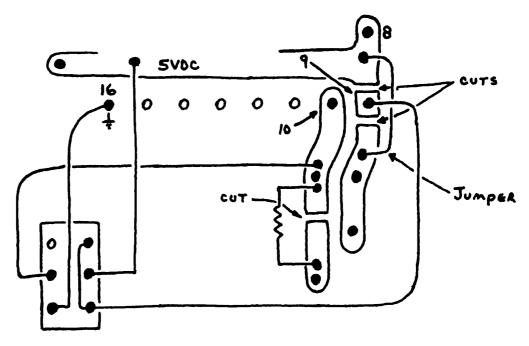
If switch is wired exactly as shown will have the following: Switch DOWN: Selector Position 1-40; 26.325 - 26.765MHz Switch UP: Selector Position 1-27; 26.645 - 26.955MHz Switch CENTER: Normal Operation..
