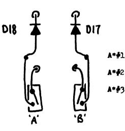
\*Remove Anode side from PCB on both D17 and D18. Solder wires to diodes and to where removed as shown. Wire switches accordingly. Fo Table below:
