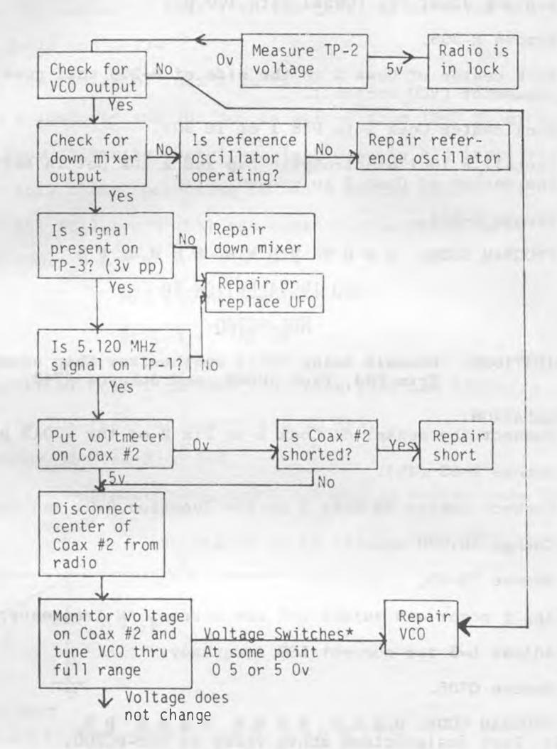
As the VCO is adjusted through the frequency displayed by the UFO, the voltage on Coax #2 should change its logic state.
