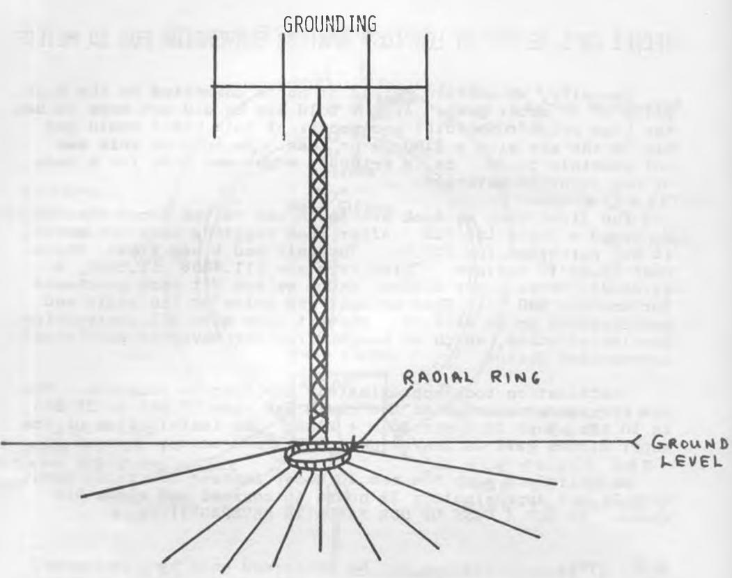
1/Radials must be at least 16 feet long and no longer than 36 feet. 2/Radials must be just below the surface of the ground or on top.
