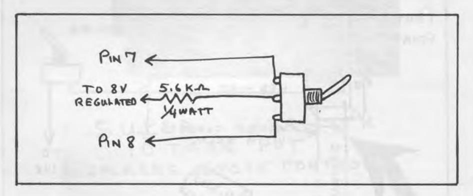
Install a SPDT Center Off toggle switch as show.
