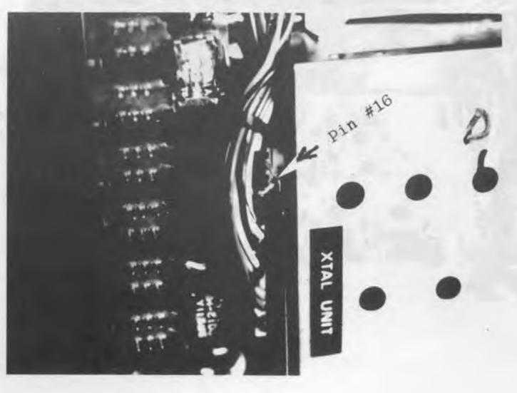
4-Remove counter box in back of display unit. The PLL unit must be removed first to allow the counter unit to be removed. Notice the colored wires soldered in the circuit board next to the two integrated circuits Y7 and Y4. Remove the blue, violet, grey, and white wires from the circuit board and re-connect them as shown, using silicon diodes in series.
