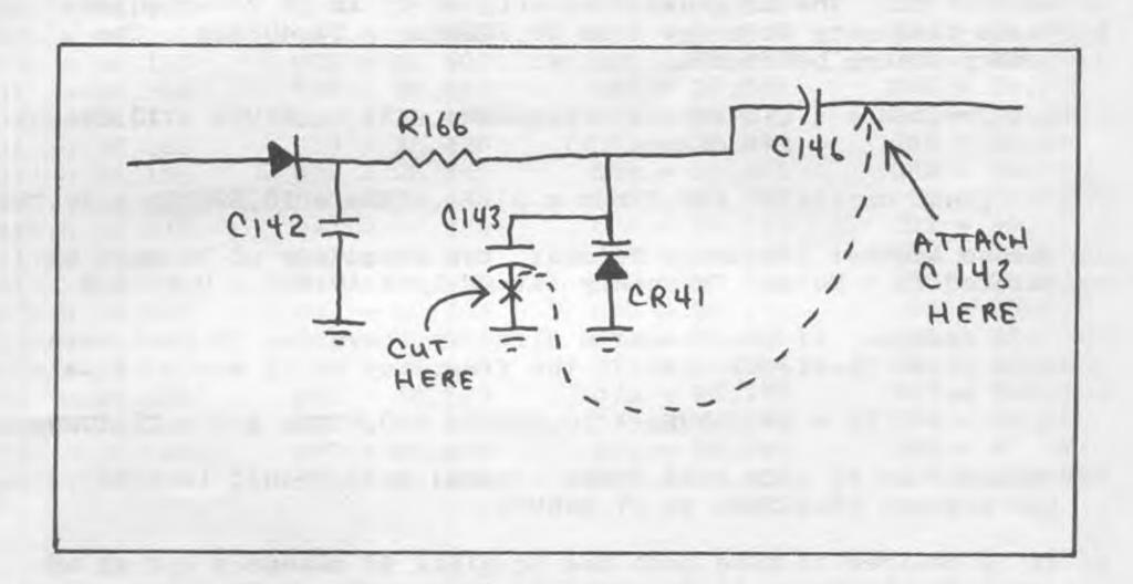
Remove C143 (10pF) and reposition it so it is wired in parallel with C146 (22pF). This will bring the frequency up several KHz. Readjust added coils for exact frequency.
