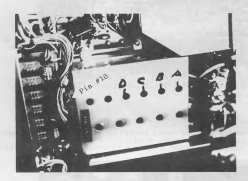
Do not remove cover of VCO unit to adjust. Make the adjustments with a small non-metallic tool.
