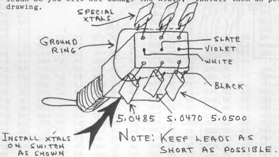
2-Mount your new switch in a convenient position thru the front panel.
