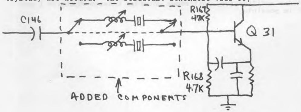
The circuit board should include the two crystals and two coils. The coil-crystal combinations are wired to the throws of the PC-C3 switch. The wipers of the switch should be wired to the original Y2 mounting holes in the 8092 circuit board. The added circuit board should be installed as close to the PA-CB as possible and with wire as short as possible to minimize frequency variations caused by stray inductance.
