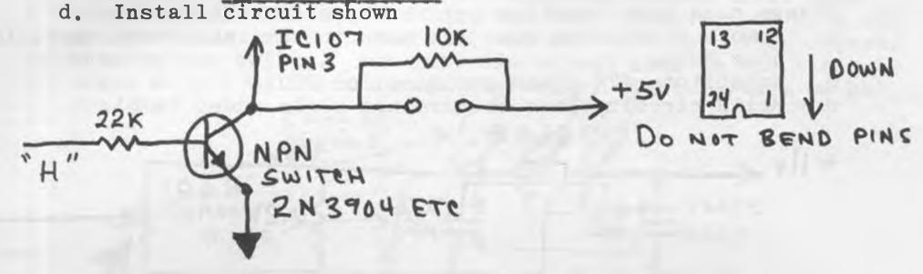
Circuit recognizes greater than 7 (HEX) and switches IC 107/3 low to add 256 to required division.
