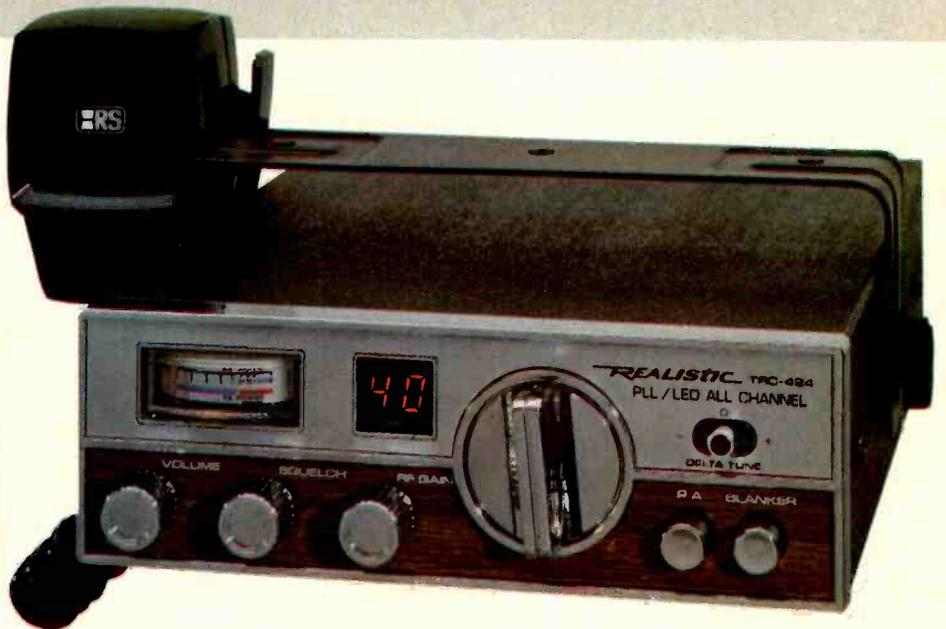
**The TRC-424** is our top-of-the-line mobile transceiver, and it's easy to see why! Switchable noise blanker—the best way to cut impulse type noise. Delta-fine tuning for pulling in off-channel stations. Adjustable RF gain. PLL circuitry and ceramic IF filters. Large LED digital readout for easy channel selection even at night. Squelch. PA capability—just add an exterior speaker. With dynamic plug-in mike, mounting bracket, power cables for 12 VDC positive or negative ground. Just 169.95\*.
