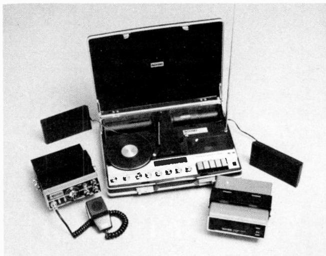
Model ARC 6100 stereo sound system contains an AM/FM radio, 3-speed phonograph and cassette tape recorder/player. Two input mic jacks provide for stereo recording from outside sources or direct recording capabilities from either the radio or phonograph directly onto the unit's cassette. This solid-state transistorized unit, with built-in antenna and two remote speakers, is both AC or battery operated. Total weight, 12 lbs. 10 oz.
