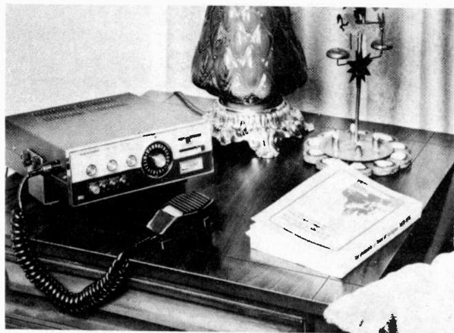
For those who feel that getting a base and mobile SSB rig runs into too heavy an outlay, at least at the start—the option is there to obtain one rig, a mobile unit, which can be used for both base and mobile use. This Realistic TRC-48 is a set which lends itself to dual use—most mobile rigs will require a separate power pack for operation on house current.
