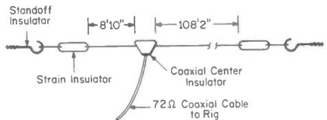
Diagram of the SIGNAL SQUIRTER — MARK I. Cut the wire of each section 2 inches longer than necessary to permit tying on the insulators.
