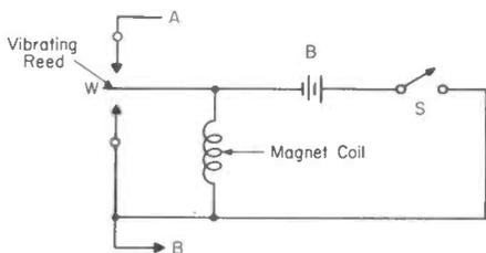
Fig. 1. Basic vibrator circuit.
