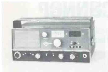
The USL Contact-8 CB Transceiver. At the bottom from left to right are: mic connector, CB-PA switch, volume control with power switch, spotting switch, receiver-tuning or crystal-control switch, channel-crystal selector, headphone jack. The squelch control is at the right of the speaker grille with the tuning dial just at the right of center. Below the meter is the meter function switch along with the two external-crystal sockets below it.
