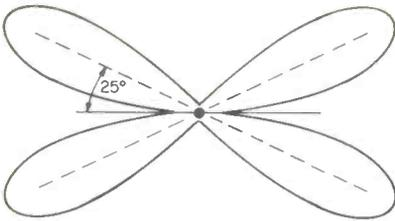
The signal pattern for the SIGNAL SQUIRTER — MARK I looks something like this, with the best signals at 25 degrees off the sides. Take this into account when you decide which direction the antenna is to be hung for maximum signal into your desired coverage area.
