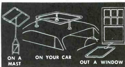
noise pickup. Not so with the horizontal antenna. Lying flat, it creates cross-polarization; noise is vertical, antenna horizontal. Electrical hash is knocked down many db.
