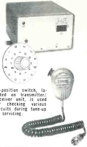
24-position switch, located on transmitter/receiver unit, is used for checking various circuits during tune-up or servicing.
