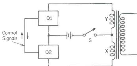
Fig. 3. Simplified transistorized power supply.
