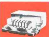
With CB channels only 10 Kc apart, selectivity is important! In the HB-500, ultra-sharp selectivity is achieved by means of a true mechanical bandpass filter in the 455 Kc IF section. At 10 Kc on either side of the center frequency, the filter provides 60 db of attenuation—an extremely high rejection ratio that assures complete adjacent channel rejection!
