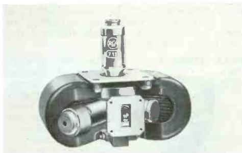
ful AM broadcast stations) and millions of watts of pulse power. Widely used in long-range radars, space research, and nuclear particle accelerators. Although the 3.5-volt filament voltage of the 7835 appears modest, the filament-current rating is a whopping 6600 amperes—more than 2300 watts for the filament alone. Price: \$7800-\$64000.
