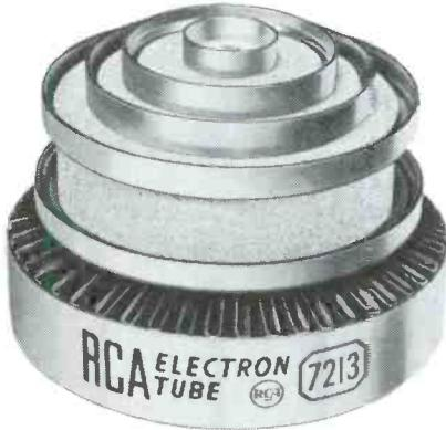
There are many families of tubes within this classification, which is flexibly defined as including tubes that produce power from approximately 15 watts to 15,000 watts. Some power tubes will be found on either side of this range. Generally, these tubes perform much the same function as the rf amplifier tube in your CB rig. Cost and size are closely connected with power-handling capability and frequency of operation. Price: \$2.50-\$2000.
