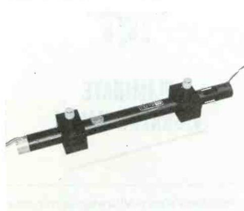
TWT's are widely used in both receiving and transmitting applications above 1000 Mc. The 7642 is a power type which delivers 18 watts at 1700 to 2300 Mc. It was designed specifically for satellite use. Price: \$900-\$3000.
