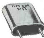
Supplied in all 23 Citizens Band frequencies. Calibrated .005%. Hermetically sealed. .486" pin spacing; .050" pin diameter; .758" height above pins; width .720"; depth .309". Be sure to specify channel desired, make and model of equipment.
