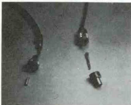
plug (the kind for auto radios) into a rig equipped with the standard coaxial socket (SO-239). The adapter shown at the left in the photo handles that job. The other unit takes care of the reverse problem—coax plug to auto-type socket. Both adapters have pin inserts and shells to properly match up connector types.
