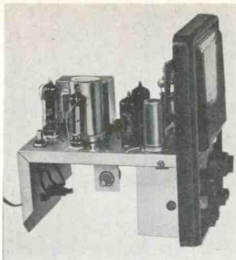
Kits with point-to-point wiring such as this EICO AC VTVM have the major components mounted directly on a metal chassis (or subassembly) and the minor parts (resistors, capacitors, etc.) wired directly to the terminals.
