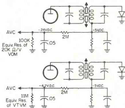
connected. Compare this against the best of the VOMs, a 20,000 ohms/volt job. For each full scale range the VOM represents the voltage times 20,000 (The five volt range is 5 x 20,000 or 100,000 ohms). The VTVM on the other hand is always 11 megohms regardless of the range in use.
