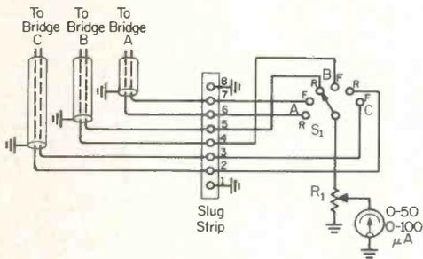
Schematic diagram of the meter box which is attached to the "thru-line" unit.
