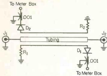
Schematic diagram of the "thru-line" portion of the SWR bridge.
