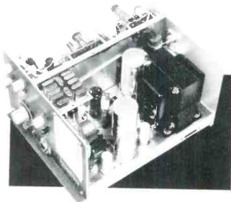
The International Model 100 Executive is designed for top performance and dependability. Here is a transceiver to fill the requirements of the most demanding Citizens licensee. Twelve crystal controlled transmit channels, a tunable dual conversion superheterodyne receiver covering all 23 channels, plus two crystal controlled receive positions are only a few of the outstanding features of the Model 100. Highest quality components and rugged construction add up to years of trouble free operation.
