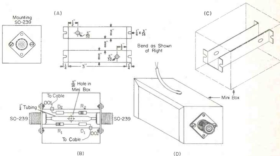
Several views of the "thru-line" part of the SWR bridge described in this article. Figures "A" and "B" show the construction of the units inner workings, Figures "C" and "D" show details of the cabinet. In figure "B," R1 and R2 are 50 to 150 ohms and matched (see text), D1 and D2 are miniature diodes (1N51, 1N34, etc., matched).
