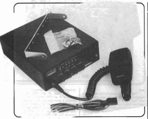
ment used to measure it! S9 on the meter measured about 60 uV and with both squelch and RF gain set at maximum, the squelch opened at 18 uV.
