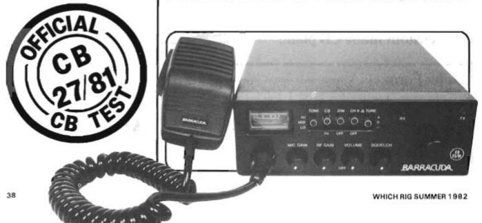
quently the dimmer switch is slightly superfluous. All the switches have a nice feel to them, but are somewhat close together for 'fumble-free' operation. The fact that they are slightly recessed doesn't help here either. Eliminating that dimmer switch would allow the remaining switches to be spaced a little better.
