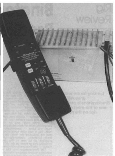
Above: Note the Hi/Lo attenuator switch on the main unit.
