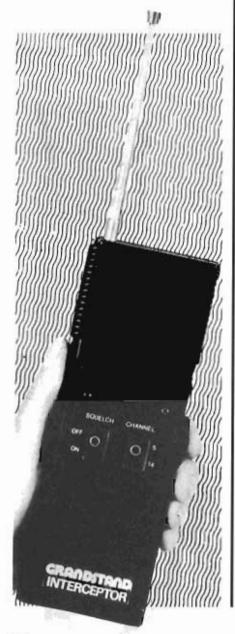
there are three rotary controls, the volume/off, the Squelch and the channel selector.
