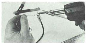
Slip the remaining part over the inner conductor and adapter, and screw on the adapter. Solder the inner conductor on the tip of the connector. Let the solder flow into the hole a little bit. Cut the inner conductor off flush with the tip.
