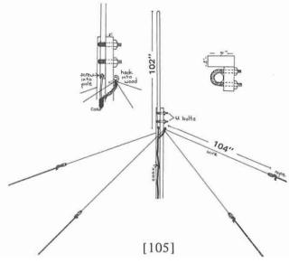
The inside conductor of the coax is connected to the aluminum pipe by means of a screw into the bottom of the pipe. See the detail drawing on preceding page. Coat this connection with sealer or cover it with tape to protect it from corrosion.
