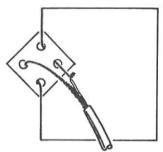
inches and attach the inner conductor of the coax to the end that will be the top of the antenna. Connect the shield side of the coax to the other end of the driven element. Twist together, solder, and tape each connection.
