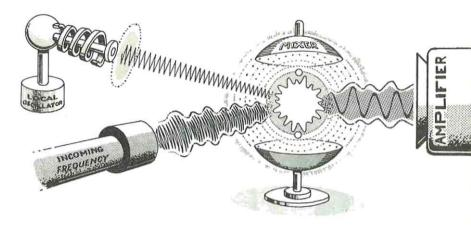
By the way, that second frequency is made by a circuit called a *local oscillator*; *local* because the signal is made right in your rig as opposed to the incoming signal which comes from tens, hundreds, or even thousands of miles away. It's also an *oscillator* because electricity oscillates back and forth in this circuit. It goes back and forth so fast that it becomes a radio frequency.
