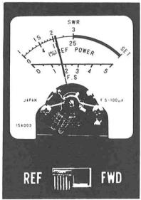
A power meter reads the amount of power that your transmitter is putting out in watts (usually about 3 watts). These meters are only accurate when used with an antenna that has a very low SWR. As with an SWR meter, the meter is connected between the output of the transceiver and the antenna. A short piece of coaxial cable, with a coax plug on both ends, is used to link the meter and the transceiver.
