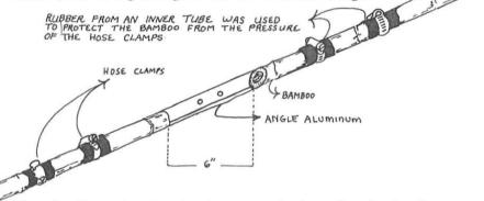
Step 3- Clamp bamboo in place on each piece of angle aluminum with hose clamps. If necessary, use rubber padding in between clamps and bamboo for a snug fit. Leave a 6-inch gap between bamboo pieces for U-bolting cross-arms to boom. The distance from tip to tip on each crossarm should be the following:
