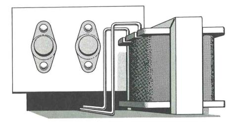
This here is the *modulator*, and it's another audio amplifier. "Modulation" is detection in reverse: we mix our voice signal with the radio frequency signal which will carry it out into the air. It doesn't matter how much we amplify an audio signal, it just won't radiate off your antenna, it's too low a frequency. That's why we need a carrier, and we'll see how it is produced in a minute.
