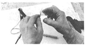
Strip outer insulation back 1¼ inches. Separate strand of braided shield very carefully; don't cut or break any of them off.
