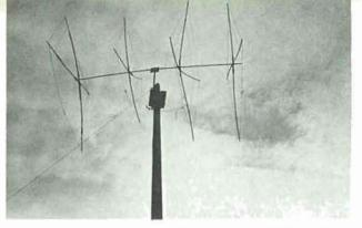
Quad Gain 2 elements = 9 db 3 elements = 12 db 4 elements = 14 db 5 elements = 17 db
