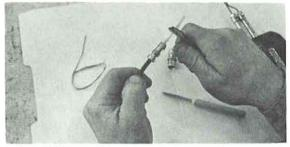
Strip the insulation off the center conductor of the coax, leaving a little more than 1/4 inch of insulation next to the adaptor.
