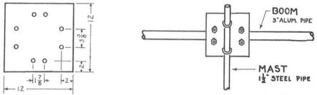
The antenna can now be mounted on the tower or pole. The mast is used between the rotator and the boom.
