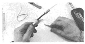
Slide adaptor up to end of black outer insulation and bend the shield down over it. Then cut the shield so that it doesn't extend down over the threads of the adaptor. (RG8 is larger than RG58 and does not require an adaptor. The braided shield is folded back on itself.)
