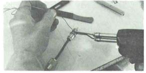
Hold soldering gun on the holes of the connector until it gets good and hot. Apply solder to the iron and hole. Don't use too much solder. You'll have to slip the outside of the connector over this solder joint. Be careful not to heat up the connector or coax cable to the extent that you melt the insulation.
