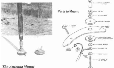
The main point to understand when making an antenna mount is that the antenna itself is not supposed to ground out to the body of the vehicle. This means that the bolt the antenna hooks to must be insulated from the metal body.
