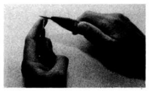
(6) Carefully cut round inner insulation without scoring inner wire or wires.
