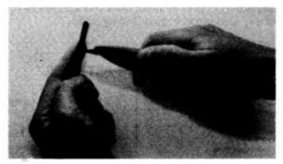
(2) Carefully cut round outer insulation without scoring braid, approx.  $1\frac{1}{2}$ " from end of cable. Rub cable against knife to cut and watch fingers!
