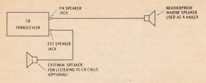
Fig. 6-2. Hook-up of a "Hailer" Speaker.
