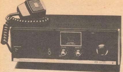
Fig. 1-1. A typical CB base station transceiver.
