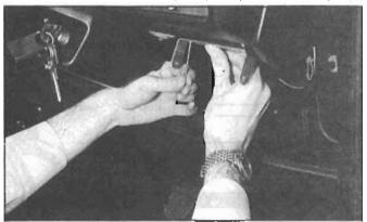
6. Work out where the mounting holes will go. Here we use a drill as the guide. Check there are no wires behind the fascia before you begin to drill the holes. The result here could be a nasty short, blown fuses, and at worst burnt out instruments!
