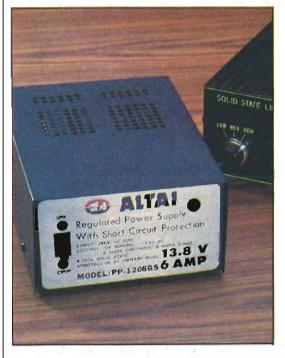
Left: The alternative to a car battery and trickle charger set-up, a 13.8v mains regulated power supply. This Altai item has the added safeguard of a short-circuit protection facility. Remember, if you do intend to use a mains transformer, make sure that it is a purpose-built CB unit, and not a left-over from your old train set!
