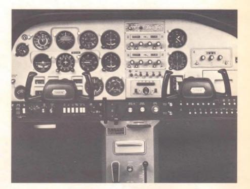
Though flight instruments make up the heart of this Cessna Cardinal's instrument panel, more than half (including the entire right-hand side) is devoted to radio or radionavigation.
