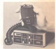
Though it looks fairly conventional, all the primary operating controls including volume, squelch, channel selection and LED readout are mounted on the microphone of SBE's Model 32 CB.
