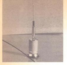
"Snap-in" mount mobile antennas can be used on rooftops where they'll provide a nearly uniform pattern in all directions or rear decks or trunk lids where they'll do almost as well. This example features a high efficiency, extra large loading coil. (Antenna Specialists)
