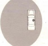
Mounting the antenna on the rain gutter gives about the same signal fore and aft, though it's strongest to the opposite side of the car.
