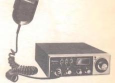
The Model CB-755 from Boman has a meter circuit to make SWR measurements.
