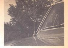
A disguise antenna has no loading coil so looks exactly like the BC antenna in whose mounting hole it fits. This helps avoid tipping rip-off artists that the car is CB-equipped. A special coupler lets it operate on both CB and the broadcast band. (Antenna Specialists)
