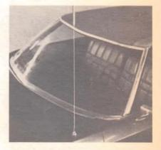
A front fender mounted CB antenna can sometimes utilize the hole drilled for the original broadcast antenna. The CB antenna is then used for broadcast reception as well as CB, either through a coupler or with a switch. (Antenna Specialists)
