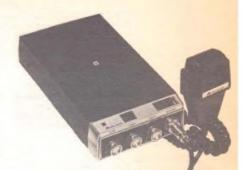
The channel indicator and meter in this Midland 13-862 are mounted at an angle for easier viewing.
