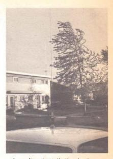
A rooftop installation is the neatest appearing, most uniform in radiation and toughest to install of all mobile antennas.
