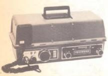
This Transcom Model 2701 has an XTAL CB transceiver plus an AM/FM tuner with 8-track tape deck and three speakers.
