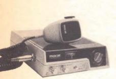
Current mobile rigs are more compact and designed to fit in with a modern auto's decor. This Motorola Mocat is designed for under-dash mounting.
