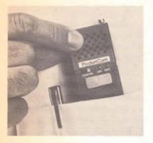
100-milliwatt 27 MHz transceivers aren't legally classified as CB rigs though they do operate on CB frequencies. Ultra compact vest pocket models like this make very convenient short range communications tools. (JS & A Sales)
