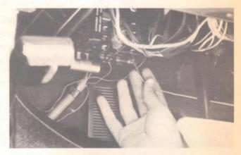
Connect the positive power lead to an appropriate spot in the fuse block. For safety's sake, it's best to disconnect the positive lead to the car battery when you're working around the fuse block.
