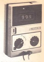
Digital multimeters like this B&K Model 280 are much more precise and easier to use than conventional VOMs and still retail for under \$100.
