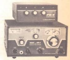
Drake's SPR-4 general coverage shortwave receiver can be digitally tuned with the FS-4 accessory synthesizer.
