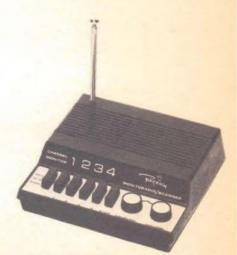
Eavesdropping on police, fire or other VHF/FM services is the current SWL rage. Regency's ACT-C4 is a 4channel scanner that covers both VHF high and low bands along with UHF.
