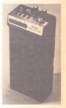
Pocket scanning receivers are also available in sizes little larger than a cigarette package. The RCA 16S100 is a 4-channel scanner that can monitor a combination of VHF and UHF frequencies.
