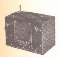
Vocaline JRC-400, probably the best known of the early (mid 1950s) commercial equipment for UHF/CB. Designed for mobile or fixed Class B use, the JRC-400 sold for under \$140.00 a pair while Class A operation required commercial equipment selling for many times that.
