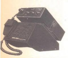
When room permits, a special hump mount like this Gambler-Johnson with built-in speaker makes a neater, more functional installation.
