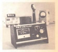
Antenna standing wave ratio meters come in a variety of shapes and sizes. Antenna Specialists' M-272 measures absolute power output as well as reflected power and modulation percentage.
