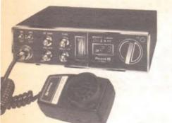
Royce's Model 1-662 features an LED channel readout with adjustable brightness and a gain control built into its mike.
