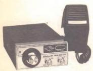
This very compact unit has a row of LED lamps instead of a meter for signal strength and output indication. (Fieldmaster)
