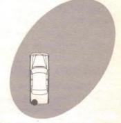
Mounting the antenna on the bumper produces a pattern even more directive toward the front and side.
