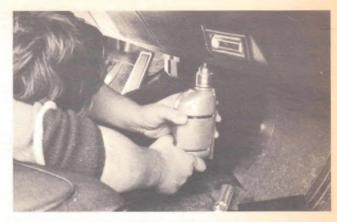
Use the mounting bracket to locate the mounting bolt holes, then drill the holes taking care not to damage car wiring or accessories behind the dash with the drill bit.
