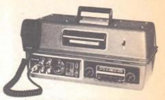
Another Transcom combines a Royce CB transceiver and separate Motorola AM/FM receiver and 8-track tape deck.
