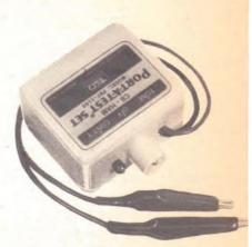
Telco's "Port-A-Test" is primarily a continuity tester—open or short circuits—but is also an "untuned" signal generator for rough checking of amplifier and receiver operation. It can also be used to indicate the presence or absence of voltage. "There are two instruments and one device that are so useful and so reasonably priced that no CBer should be without them. These are the multimeter, the antenna standing wave ratio meter and the dummy load."
