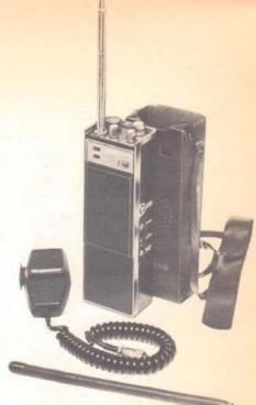
Midland's 5-watt, 6-channel transceiver can be used with a speaker/microphone, features a jack for an external antenna and top-mounted controls. Note optional flexible ''rubber ducky'' antenna.
