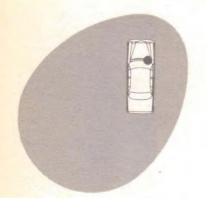
Cowl mounting puts the maximum signal to the rear and over the opposite fender.
