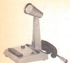
Accessory base station mikes offer more features than those usually supplied as original equipment and are almost a must when a mobile rig is used as a base station. This example from Midland has a locking push-to-talk switch and built-in pre-amplifier.
