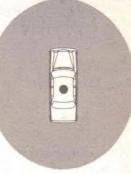
Putting your antenna at the center of your car roof provides the most omnidirectional coverage.
