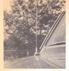
Antenna Specialists' MR 264 looks like any ordinary broadcast whip though it's actually a dual purpose CB/BC antenna. It utilizes a special coupler that enables it to function on both AM and FM broadcast reception at the same time it's being used on CB.
