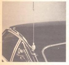
For hatchbacks a ''no-hole'' mounting bracket that can be adjusted to make the antenna vertical is available. (Antenna Specialists)
