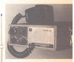
Pearce-Simpson's Capri 25 not only covers the necessary VHF marine channels but also includes both VHF weather channels and a broadcast band receiver.
