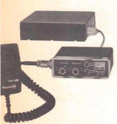
Royce's remote mount radio has channel selection and indication on the microphone, other controls on the control head.
