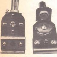
Detail of semi-permanent gutter mounts. (Antenna Specialists)
