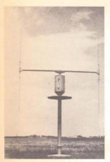
Adcock direction finding antenna used by FCC monitors to pinpoint illegal stations or locate vessels in distress.
