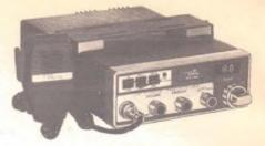
An LED channel indicator highlights the Regency Model MT-55 synthesized marine radio which covers all 55 domestic and international marine FM channels.
