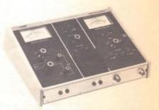
One of the more ingenious CB service ideas to come along is B&K's 1040 **Servicemaster**. With the addition of only a signal generator, it checks out all of a CB set's operating parameters.
