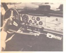
By far the majority of CB mobile rigs are simply bolted under the dash like this Standard. Note that the radio is far enough to the right that the mike coil cord clears the steering wheel.
