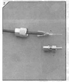
Connecting a PL529: 1. Outer braiding has been exposed and combed back. 2. Outer half of the PL529 is pushed back over co-ax once inner cable has been stripped.
