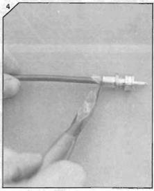
Once your RG58 co-ax has been threaded through PL529, inner wire should be secured by delicate soldering at tip of connector.
