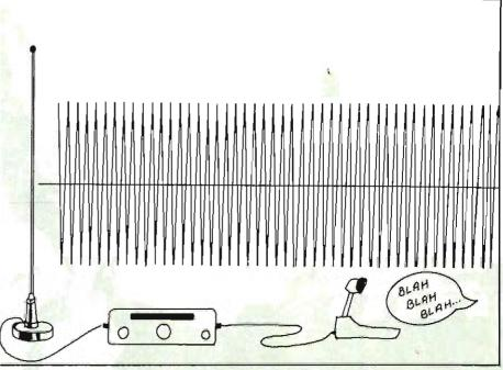
Above: The unmodulated radio wave, ie without speech or any other normal sound. The wave is symmetrical to the centre line so the crests are equidistant between each other and the centre line. This is how the wave appears (il you could actually see it), leaving the antenna. Otherwise known as a carrier wave.
