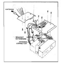
Top: All the weight of the rig and its mount is taken by these screws, therefore make sure they have a good grip and won't work loose.
